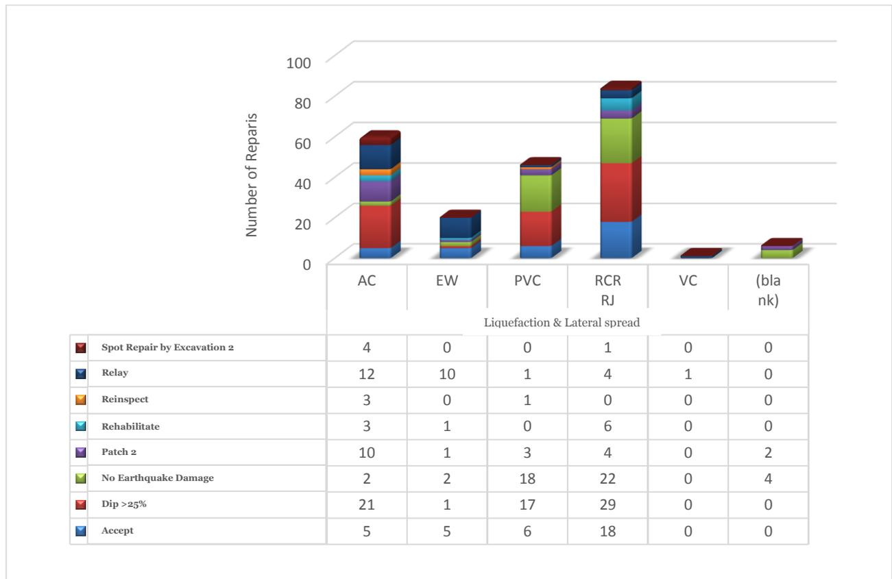
Figure 4-3: Works to Reinstatement Condition in Areas of Liquefaction or Lateral Spread
