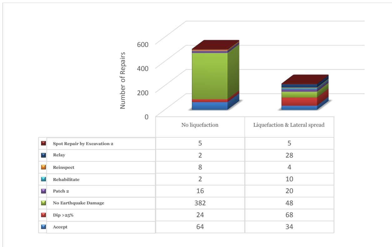
**Figure 4-1: Total works Required to Reinstatement to Pre-Earthquake Condition**
