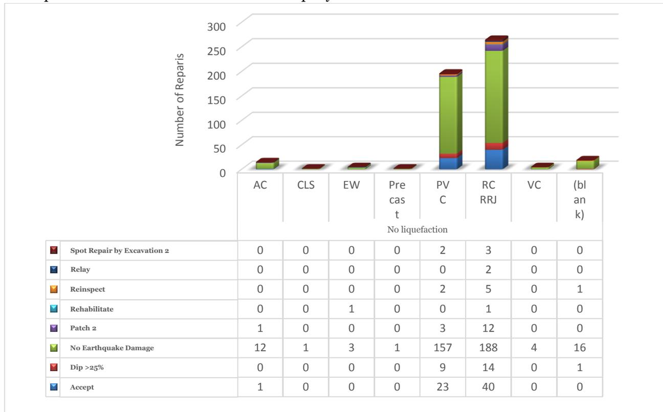
Figure 4-2: Works Required to Reinstatement to Condition in Areas that did not liquefy
