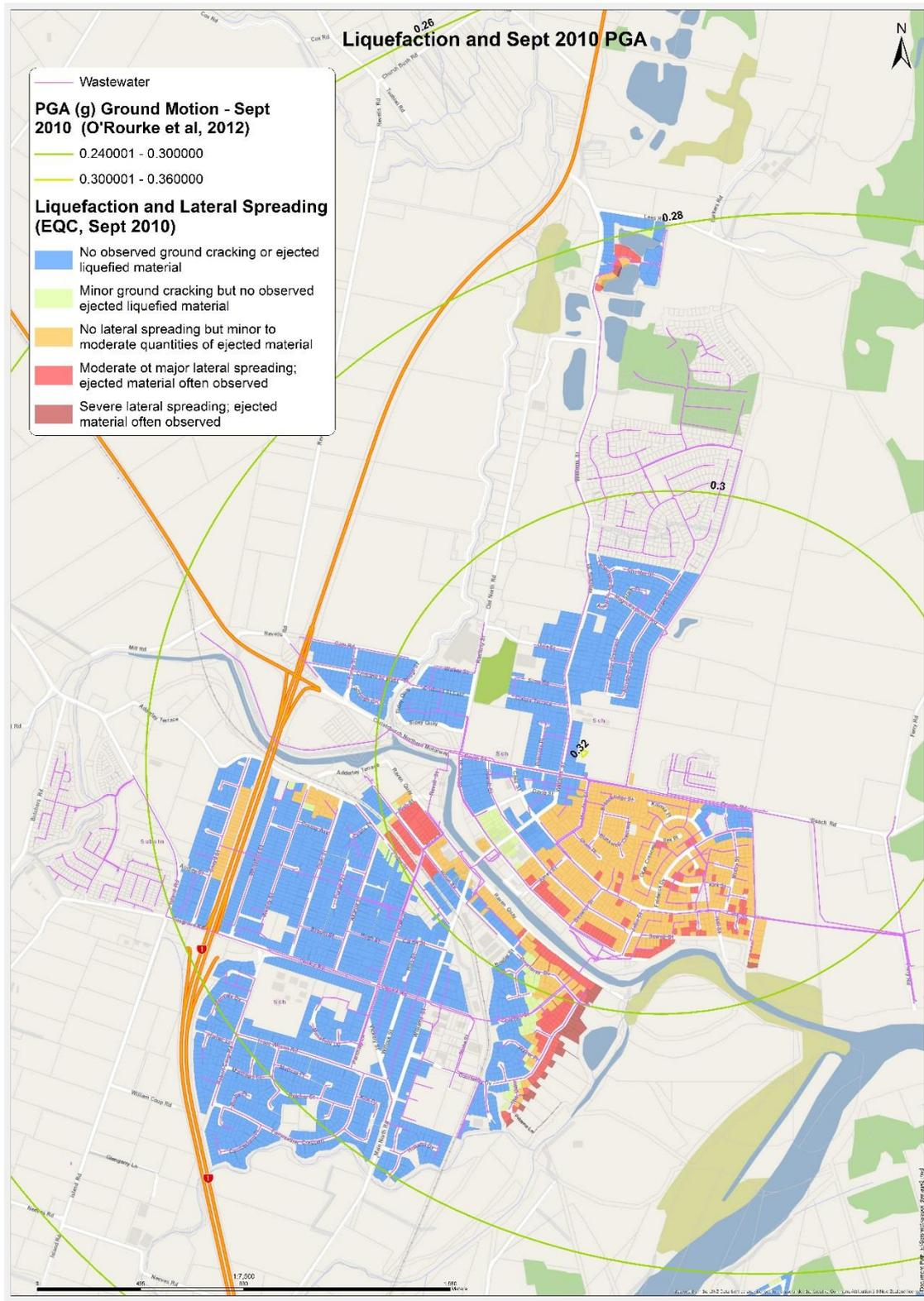
**Figure 2-2: Kaiapoi Wastewater Network and Peak Ground Accelerations and Liquefaction and Lateral Spread Resulting from the Darfield Earthquake**
