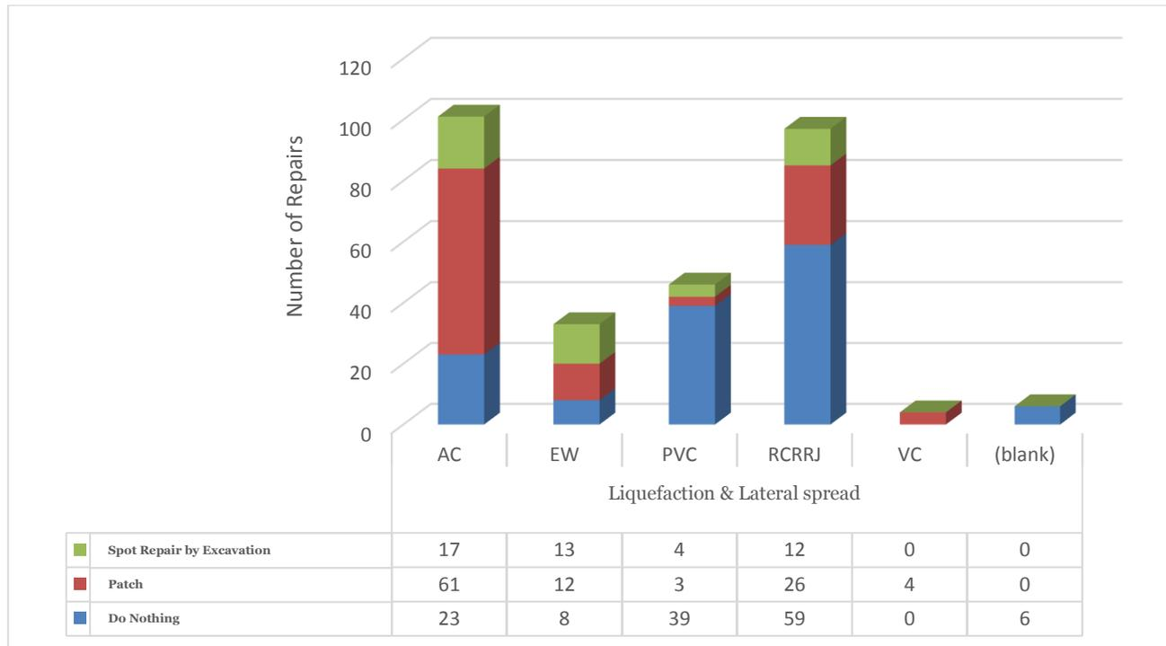
Figure 3-3: Restoration Works in Areas Where Liquefaction or Lateral spread occurred
