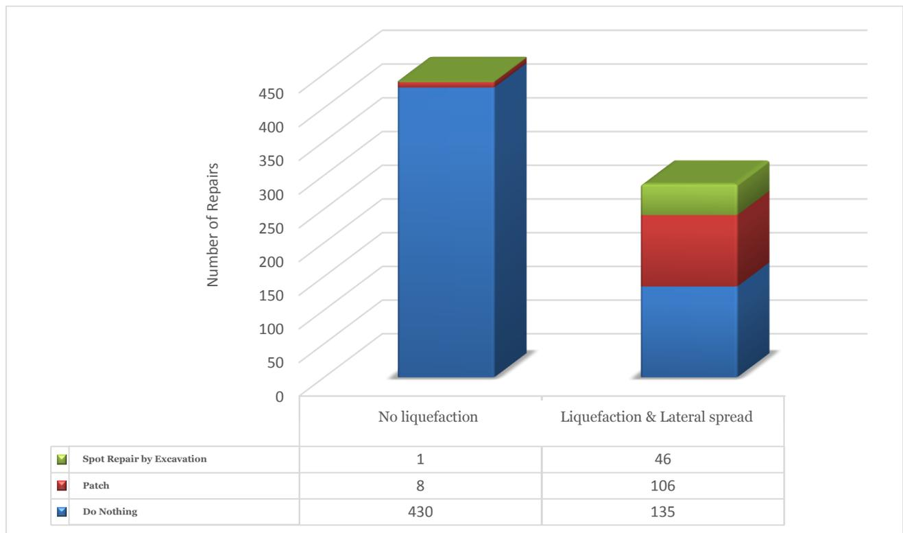
Figure 3-1: Restoration Works (Based on Liquefaction Areas Recorded by Tonkin & Taylor)
