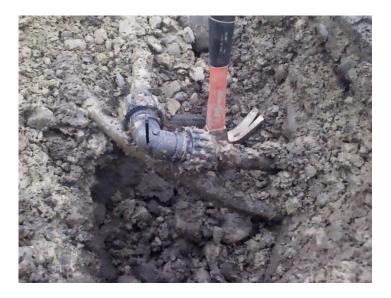
Reference: FT007 Material: PE Description: Compression fitting failed. Cause: Ground movement Repair: Replace damaged fitting
