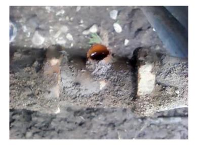
Reference: OT08 Material: Copper Description: Copper pipe failed. Cause: Unknown, possibly PGD Repair: Replace damaged fittings Comment: Modern service pipe materials with inserts in mechanical joints would perform better.
