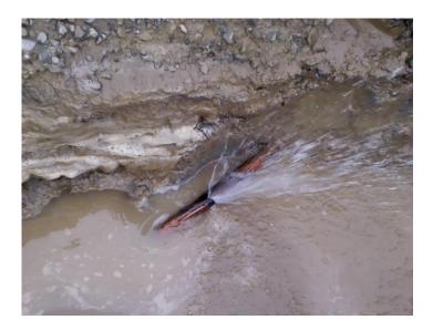
Reference: Pl005 Material: Copper Description: Crack
