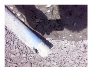
Reference: EX005 Material: PE Description: Break Cause: Probably interference damage.
