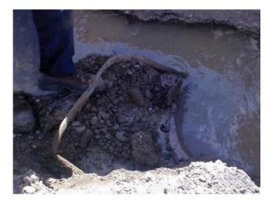
Reference: PI004 Material: Copper Description: Bending Cause: Compression
