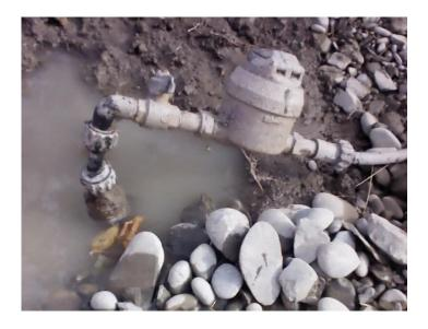
Reference: OT009 Material: PE Description: Displaced joint. Cause: Ground movement. Repair: Remake joint. Comment: While modern PE with ins
