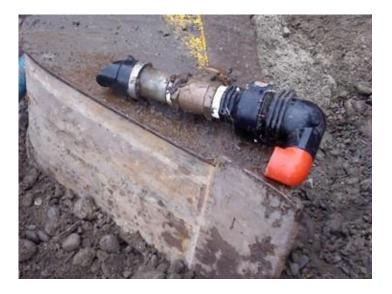
Reference: FT010 Material: PE Description: Compression fitting failed.
