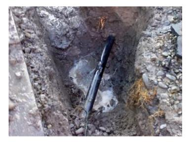
Reference: PI015 Material: PE Description: Buckling Cause: Compression
