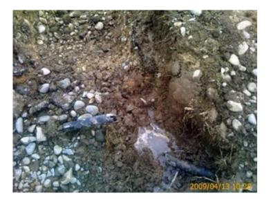
Reference: PI025 Material: PE Description: Pipe failed. Cause: Tension and lateral displacement. Repair: Replace damaged pipe.
