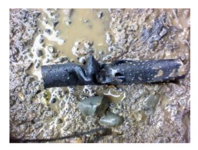
Reference: PI013 Material: PE Description: Buckling and tear. Cause: Compression
