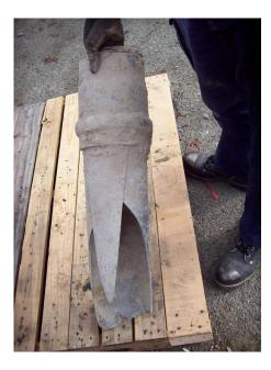
Reference: EX009 Material: PVC-U Description: Break Cause: Impact during shaking or PGD. Repair: Replace damaged pipe.
