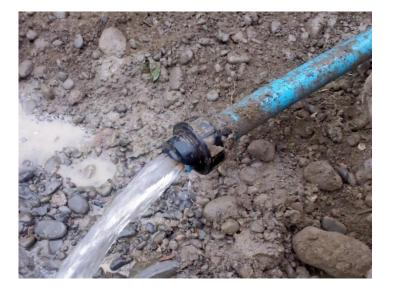
Reference: FT006 Material: PE Description: Compression fitting failed Cause: Ground movement
