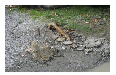
Reference: PI008 Material: Galvanized steel Description: Bending Cause: Compression of shallow buried pipe. Repair: Replacement
