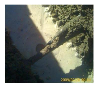
Reference: PI022 Material: PE Description: Pipe failed. Cause: Tension Repair: Replace damaged pipe.
