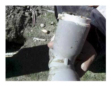
Reference: OT021 Material: PVC Description: Split elbow. Cause: Shaking Repair: Replace failed elbow.
