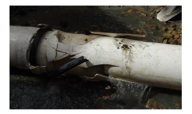
Reference: OT014 Material: PVC-U Description: Break Cause: Crushed by compression.
