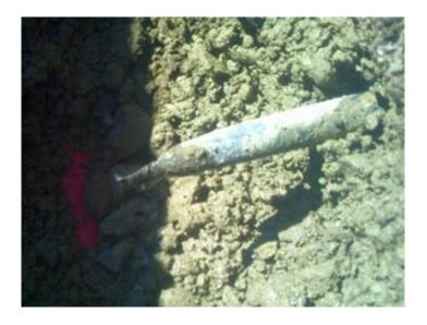
Reference: PI026 Material: PE Description: Pipe failed. Cause: Tension
