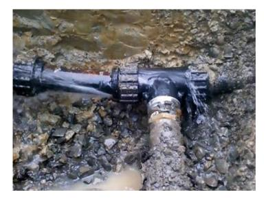
Reference: FT004 Material: PE Description: Compression fitting leaking. Cause: Tension or bending Repair: Replace damaged fitting.
