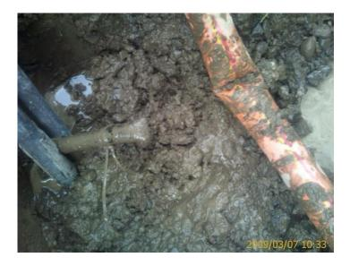
Reference: PI028 Material: PVC Description: Bending Cause: Compression of shallow-buried duct. Repair: Replace.
