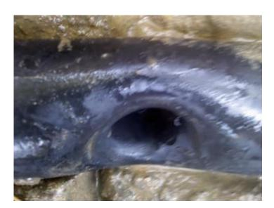
Reference: OT012 Material: PE Description: Pipe strike. Cause: Third party. Repair: Replace damaged pipe Comment: Good installation practice including warning tapes and detection wires will reduce the risk.
