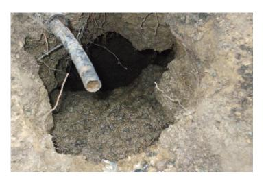
Reference: PI024 Material: PE (probably older PE) Description: Pipe failed.
