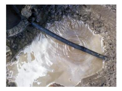
Reference: PI019 Material: PE Description: Buckling and tear.
