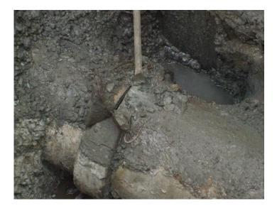
Reference: J008 Material: Concrete, reinforced Description Joint failure. Cause: Lateral shear or bending Comment: Modern pipeline systems may be more tolerant.
