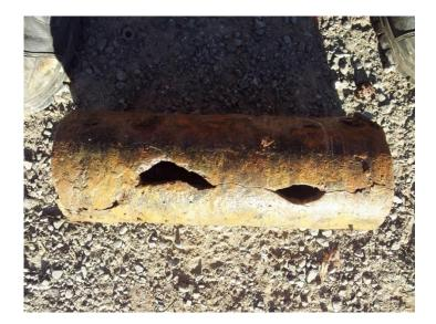
Reference: EX003 Material: Cast iron Description: Crack, holed Cause: Pressure related split.
