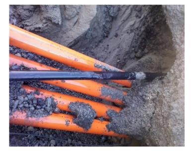
Reference: PI012 Material: PE Description: Buckling Cause: Compression
