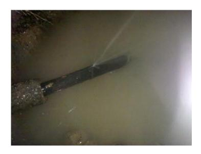
Reference: EX010 Material: Galvanized steel Description: Crack Cause: Bending or buckling. Comment: Leaking steel pipe next to coupling.
