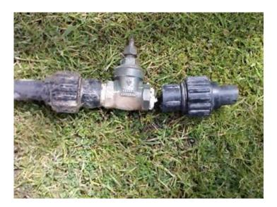
Reference: FT011 Material: PE Description: Threaded fitting failed. Repair: Replace damaged fitting.
