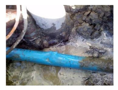
Reference: PI016 Material: PE Description: Buckling Cause: Compression Comment: Most alternative materials would also
