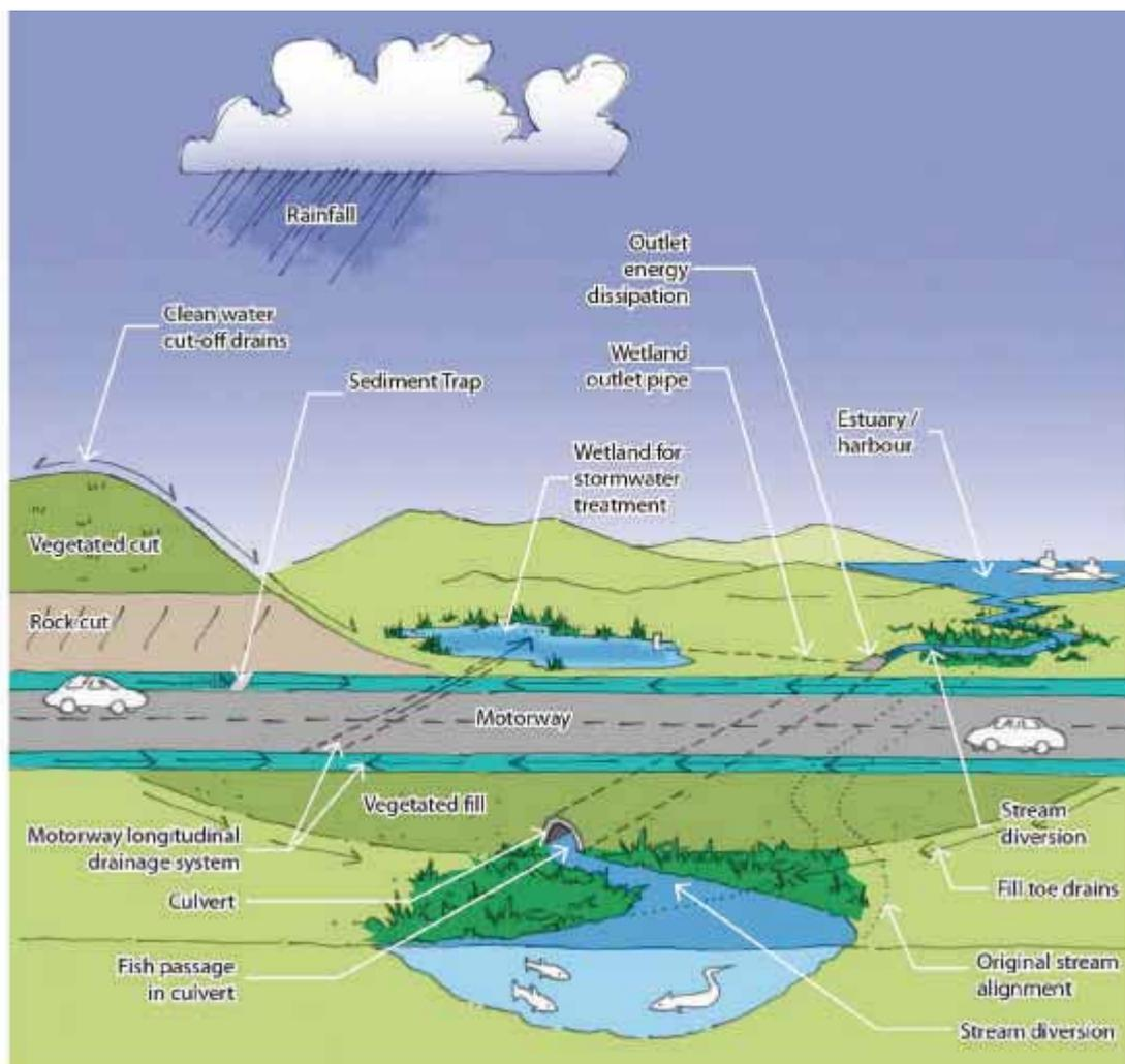
Figure 3 – Motorway Operational Water Systems and the Environment
