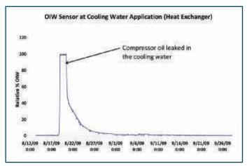
Figure 18 - Real-life oil leak from heat exchanger
