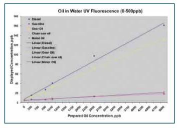
Figure 3 – Calibration curves for series of available oil products in water
