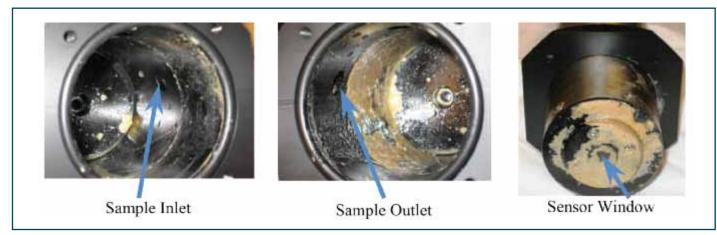
Figure 19 - After-test inspection of the flow cell and sensor window
