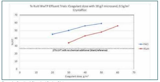
Figure 1 – Results of Chemical Dosing Trials
