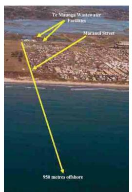
Line of landward effluent pipeline and marine outfall – Tauranga City photo
