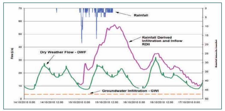
Figure 1 - Sample I/I Flow Components (WSAA Wastewater System Inflow/Infiltration Management Good Practice Guideline Document)
