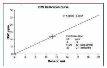
Figure 15 - Industrial WW test - calibration
