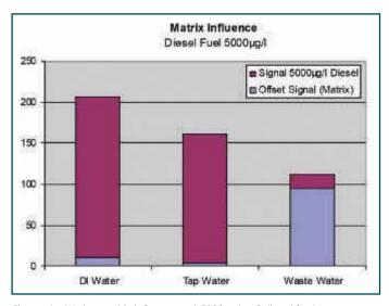
Figure 6 – Water matrix influence at 5000ppb of diesel fuel concentration
