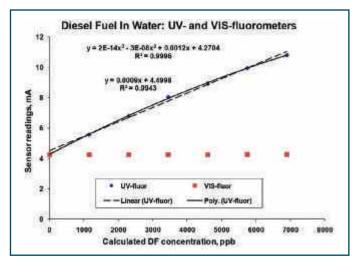
Figure 4 - UV-fluorescence: Diesel fuel calibration test results
