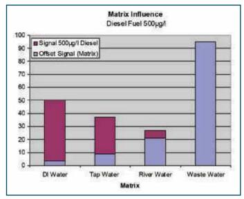
Figure 5 – Water matrix influence at 500ppb of diesel fuel concentration
