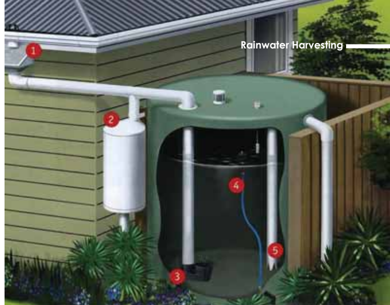
Figure 1 – Screened rainhead, first flush diverter, calmed inlet, floating out-take and tank vacuum device
