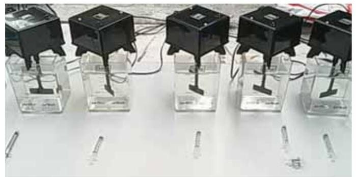
Selected results from various benchtop work are given in Figure 4 and Figure 5. Utuhina Stream results show that alum is slightly more effective than ferric chloride for control of DRP when the dose exceeds 0.5ppm. There is little merit in dosing the Utuhina Stream with much more than 1.0 to 1.5 ppm Al<sup>3+</sup>. At these rates greater than 70 percent binding of DRP onto aluminum can be expected.
