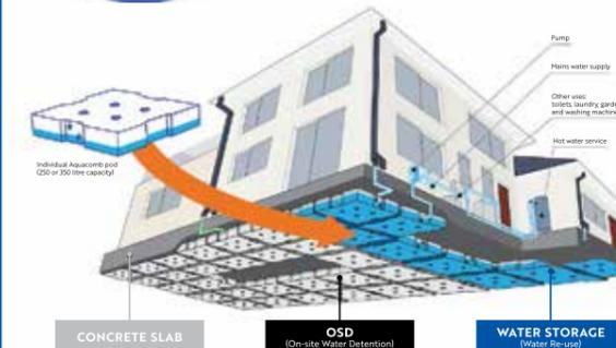
CONCRETE SLAB OSD (On-site Water Detention) WATER STORAGE (Water Re-use)
