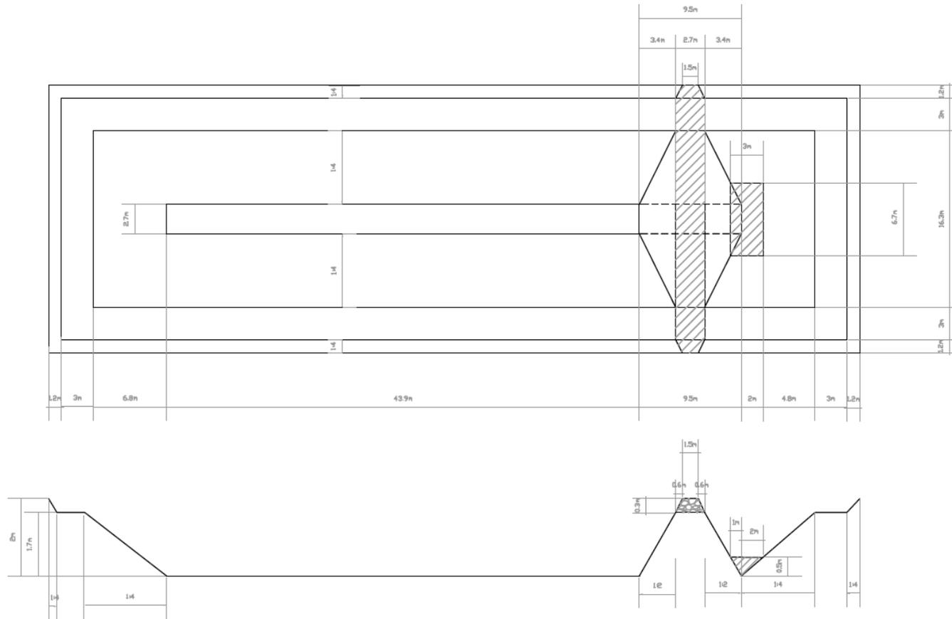
Figure 4-2 Bathymetry and computational mesh for pond detailed in Figure 4-1.
