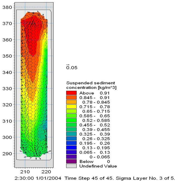
Figure 3-3 Plan View 1:1 Aspect Ratio: Suspended sediment concentration and flow vectors at mid-depth.
