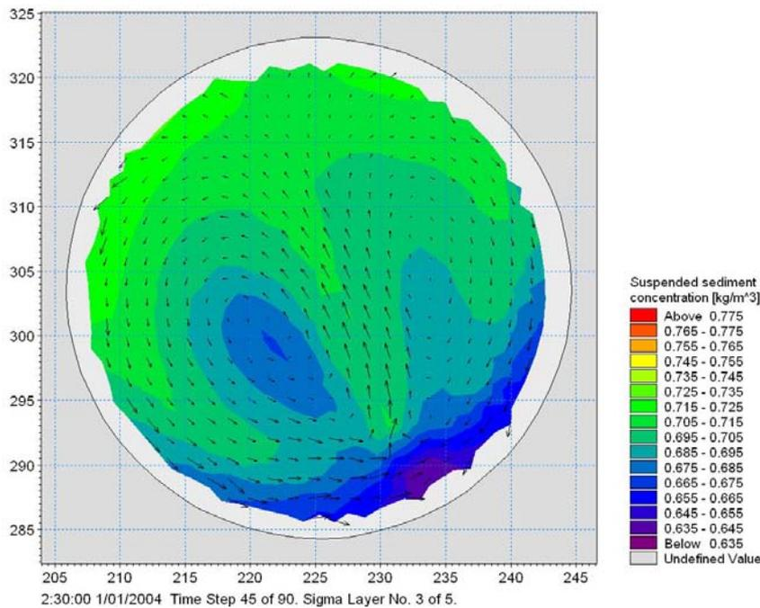
Figure 3-6 Round Pond; Inlet 20 degrees from outlet, pointing 30 degrees from tangent. Sediment concentration and velocity vectors at mid-depth
