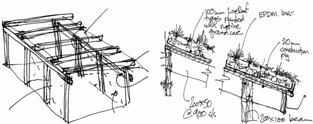
Figure 6: Carport and Live Roof Detail.
