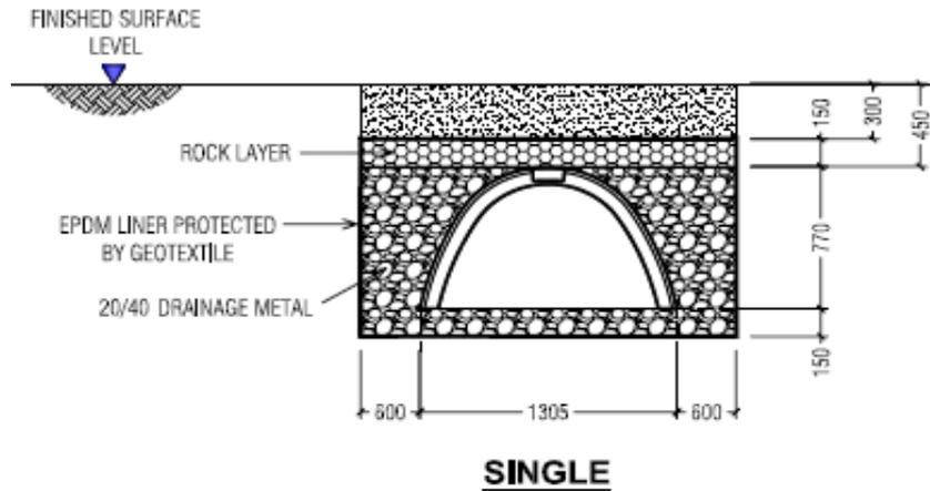
Figure 3: MaxxTank Elevation
