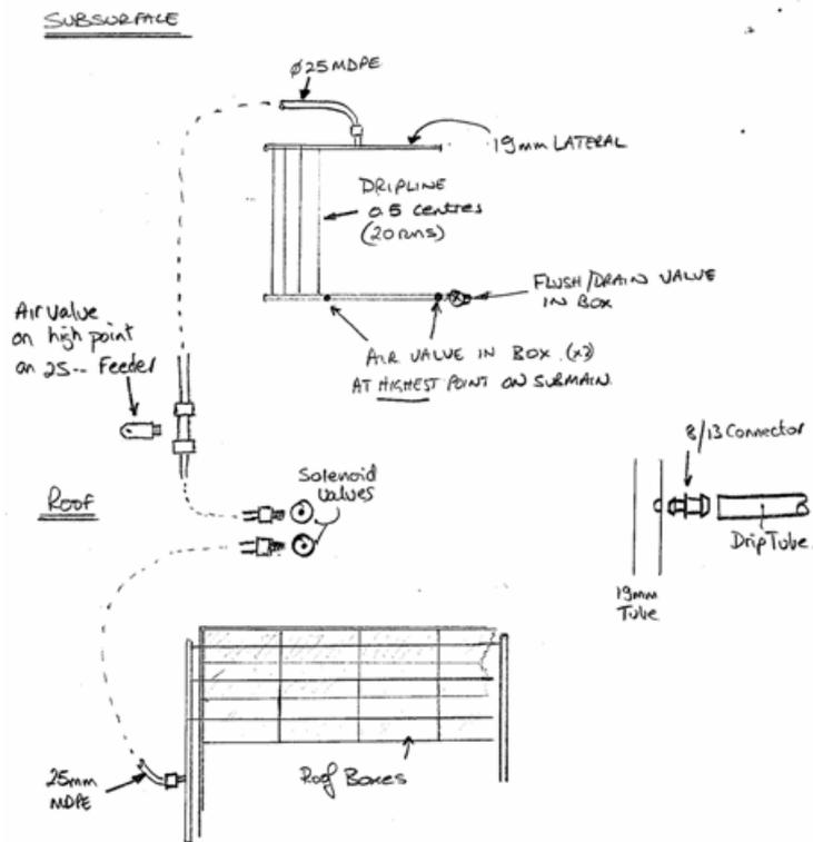
Figure 5: Irrigation Schematic
