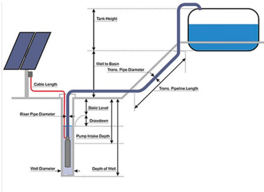
Figure 4: Solar Pumping System Schematic
