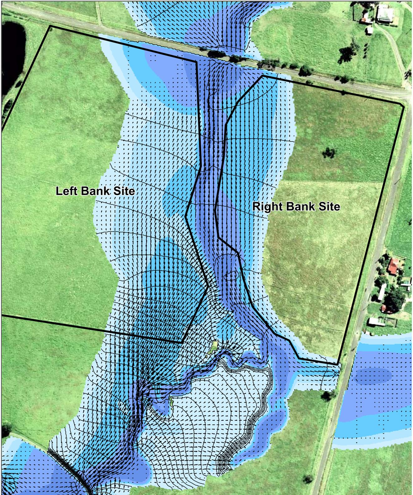
Figure 1: The flood depths using darker shades of blue for deeper areas, velocity of the water using scaled arrows, and black lines for water level contours at 0.2m increments.
