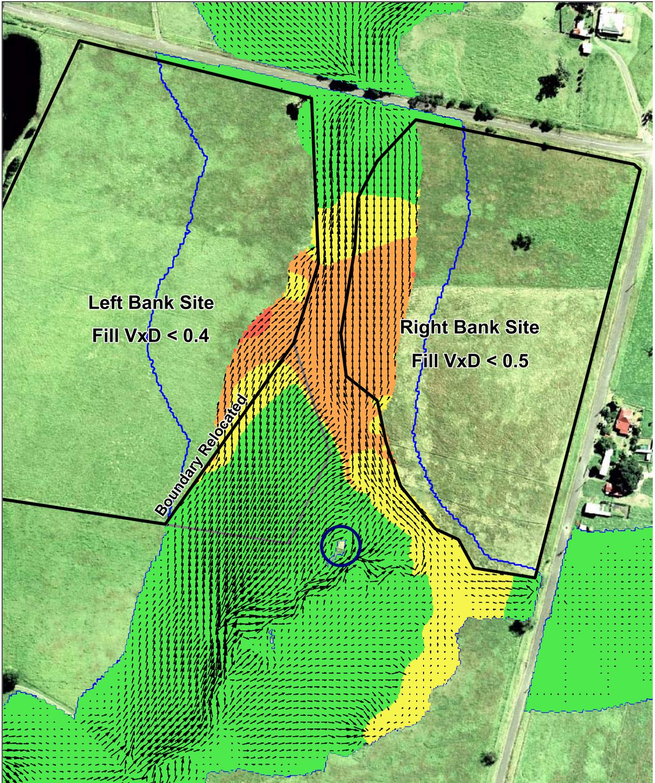
Figure 6: A possible final solution. The region for the Left Bank Site has been relocated to remove the increase along the southern boundary, and a limit of  $VxD$  of 0.4 has been set for locating fill. For the Right Bank Site a  $VxD$  limit of 0.5 has been set. The only increase exceeding 15cm (red shade) is confined on-site midway along the Left Bank Site. Increases within the waterway are all less than 15cm and the increase at the building is less than 5cm.
