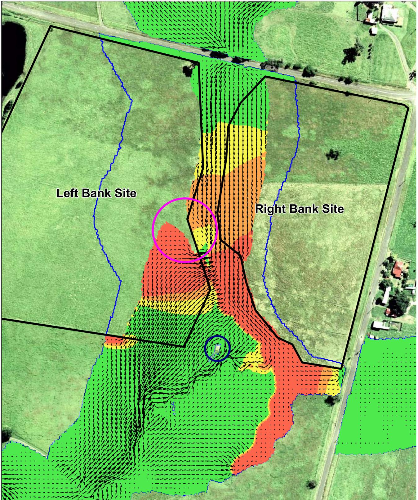
Figure 5: The flood effect of filling areas with a  $VxD$  less than 0.5. This causes unacceptably high increases in the levels within the waterway banks, primarily caused by the finger of land within the magenta circle that is blocking overland flows. The unacceptably high increase on the southern boundary of the Left Bank Site remains. The increase at the building has remained below 5cm.
