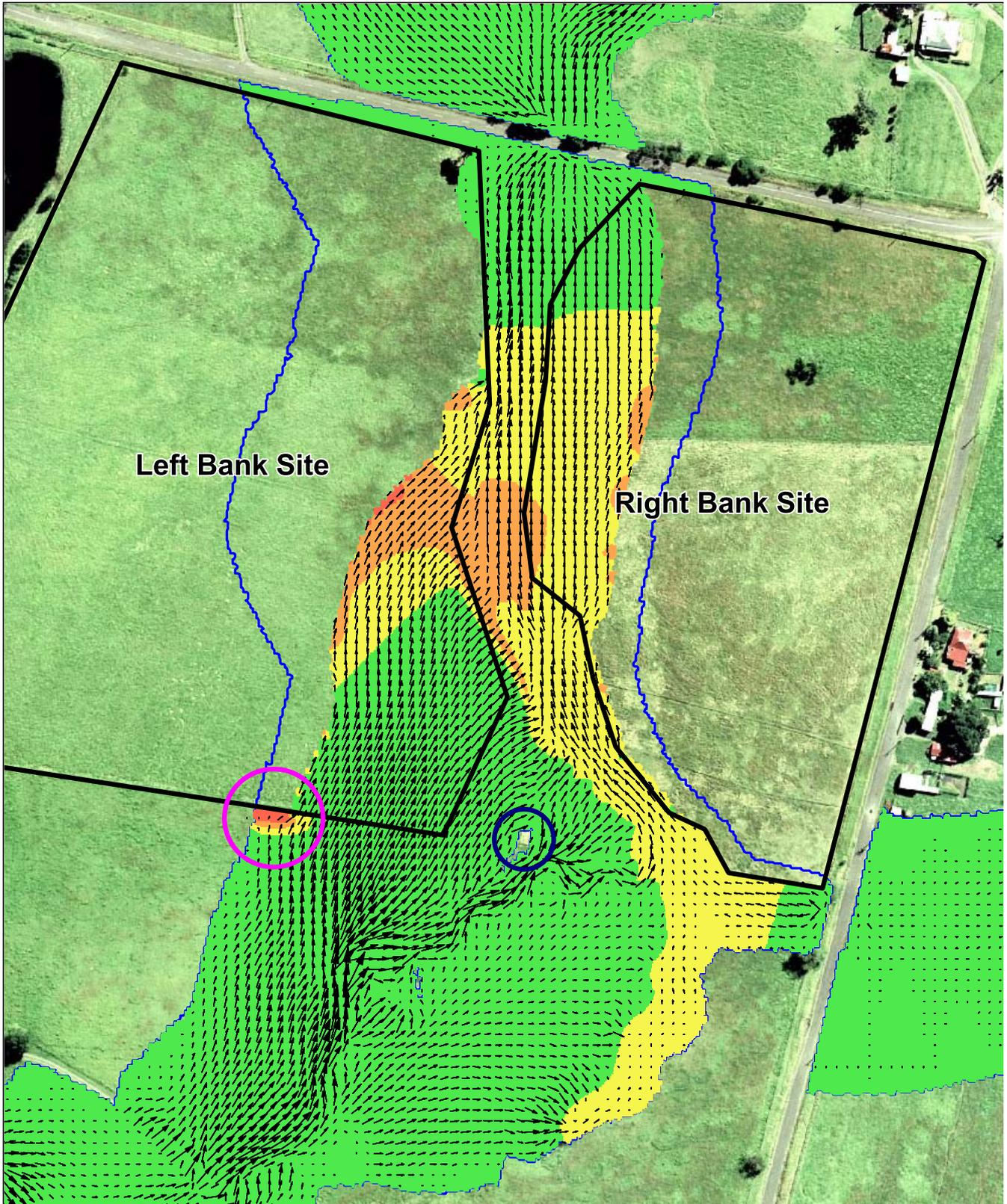
Figure 4: The changes to peak flood levels if only areas that have an existing  $VxD$  value of less than 0.4 are filled. The increase at the building is acceptable (less than 5cm) the increases within the in-bank waterway are acceptable being less than 15cm. There is an unacceptable increase in levels at the southern boundary of the Left Bank Site as circled in magenta. The original flood extent is shown by the pale blue shades and blue line.
