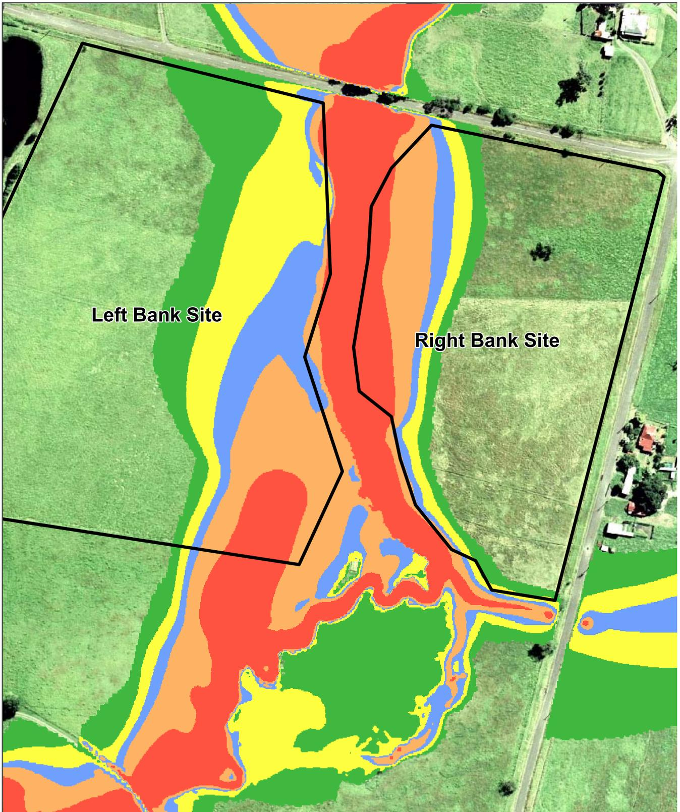
Figure 2: Map of the VxD product. Green areas are VxD less than  $0.1\text{m}^2/\text{s}$ , yellow from  $0.1$  to  $0.3$ , blue from  $0.3$  to  $0.5$ , orange  $0.5$  to  $1.0$  and red greater than  $1.0$ . Floodways will lie within the higher values (eg. red areas) and the Flood Fringe will be in the lower values (eg. green/yellow areas).
