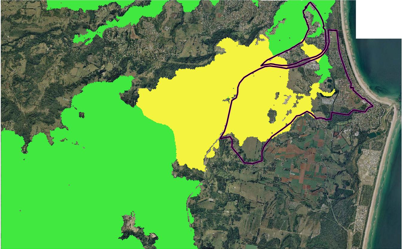
Figure 10: Increase in Q100 flood levels if only those areas with a VxD of less than  $0.3\text{m}^2/\text{s}$  within the two regions in a Q500 event are filled.
