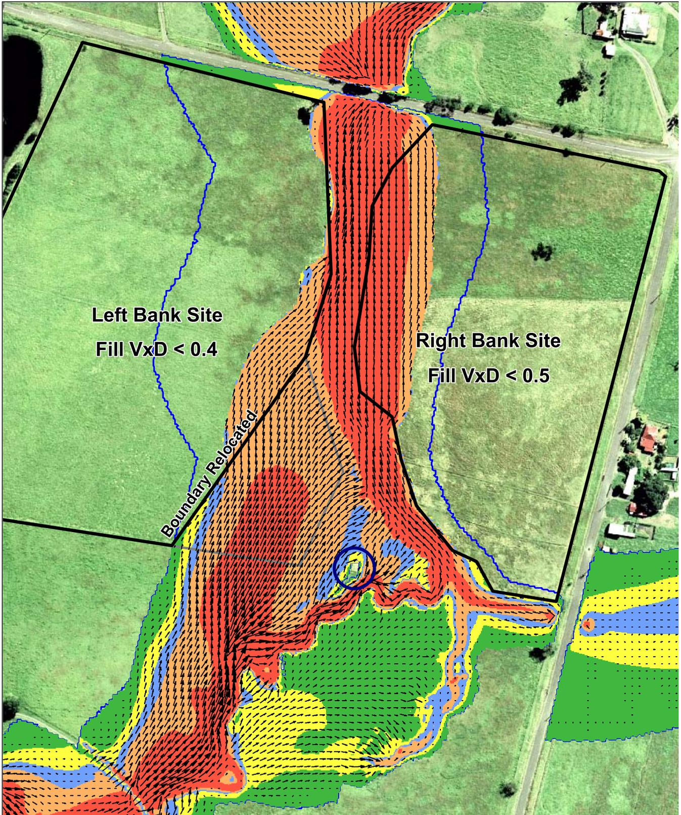
Figure 7: The VxD mapping for the final solution adopted. As can be seen, between the developments there is little green or yellow shading representing low VxD areas. The entire floodplain between the filled areas should now be classified as Floodway due to the high VxD values (orange and red shades).
