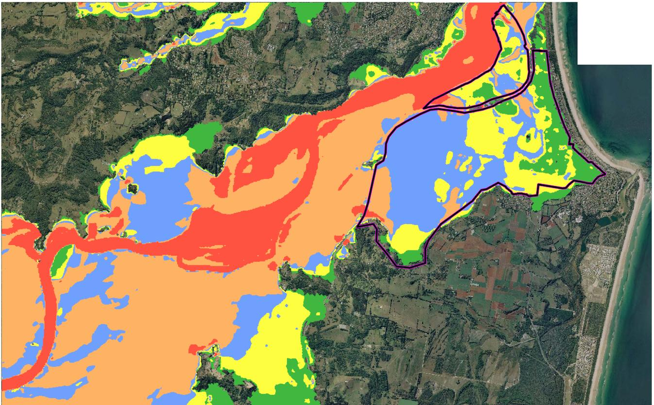
*Figure 8: The VxD mapping based on the Q500 event for the Tweed River. Green shades are for VxD less than  $0.1\text{m}^2/\text{s}$ , yellow for 0.1 to 0.3, blue for 0.3 to 0.5, orange 0.5 to 1.0 and red for greater than 1.0. Floodways would typically be red and possibly orange shades, with Flood Fringe typically green and possibly yellow shades.*
