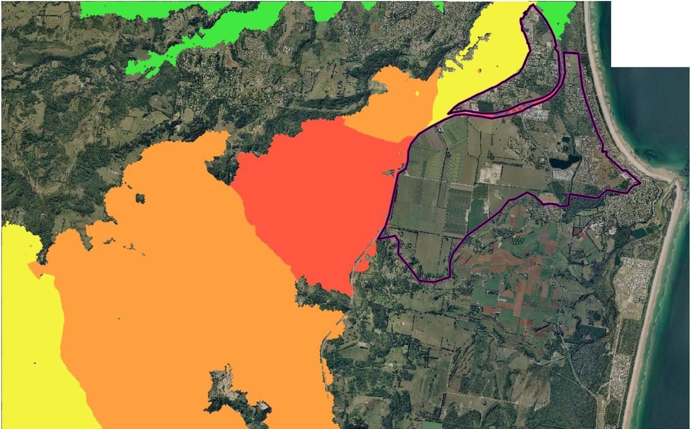
*Figure 9: The impacts on Q100 flood levels if the two regions shown in pale magenta are filled. The green shade is less than a 5cm increase, yellow 5 to 10cm increase, orange 10 to 15cm, and red is greater than 15cm.*
