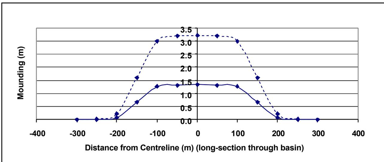
Figure 7: Predicted mounding using radial flow equation (solid line) using 2-D equation (dashed line)
