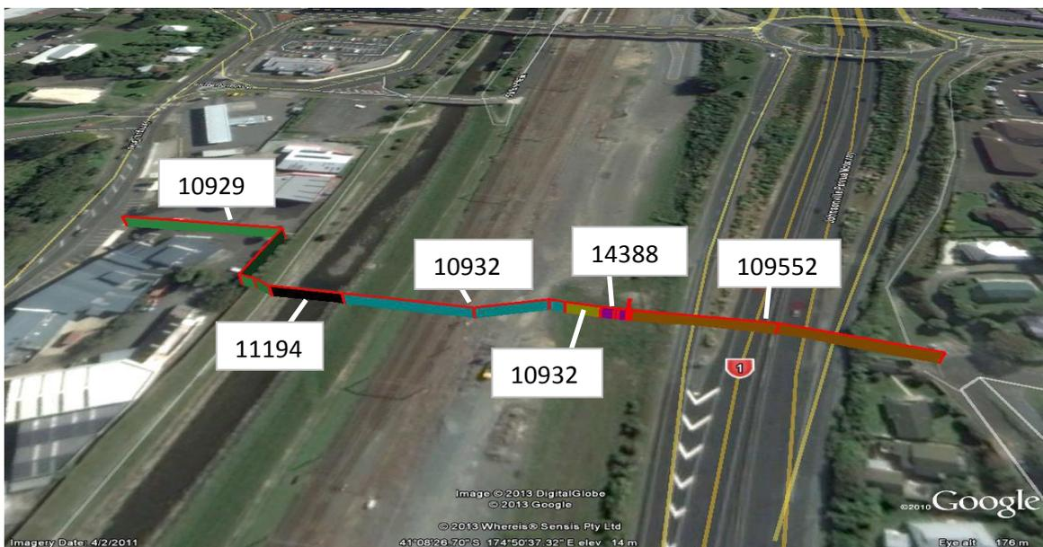
**Stretch of pipeline to be relined:** *The Photo shows the reline underneath the state Highway 1 before it continues on under the rail lines, the Regional Council stop banks and Porirua Stream*
