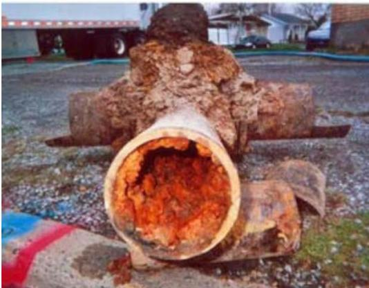
**Figure 9: Water Main Before Cleaning**
