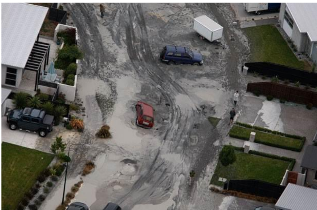
Figure 3: Liquefaction ejecta in a suburban Christchurch Street in the suburb of Bexley, approx. 10 km from the epicentre after the magnitude 6.3 Christchurch earthquake of 22 February 2011. (Photo: NZ Herald)
