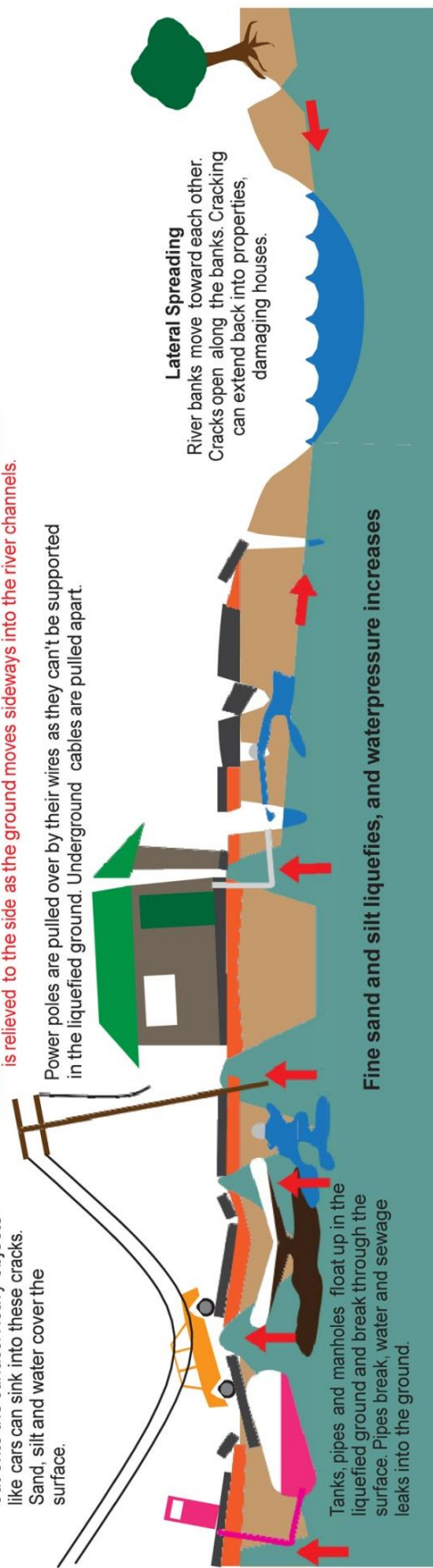
Figure 1: Diagrammatic illustration of liquefaction and its effects (IPENZ, 2012)
