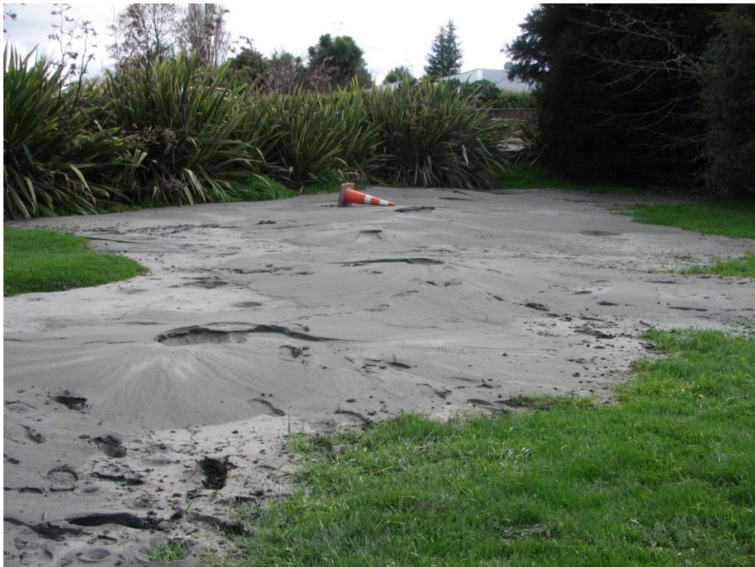
Figure 2: Sand boils caused by liquefaction in Kaiapoi, 45 kilometres from the epicentre of the magnitude 7.1, 4 September 2010 Darfield earthquake. (Photo: N. Litchfield, GNS Science)
