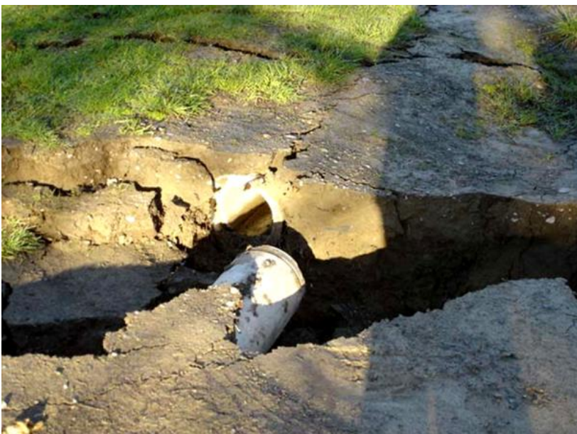
Figure 4-6. Pipe failure under tension in area of lateral spread
