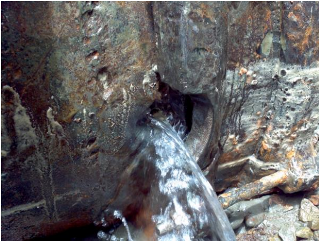
Figure 4-9. Steel pipe leaking due to dislodgement of corroded material
