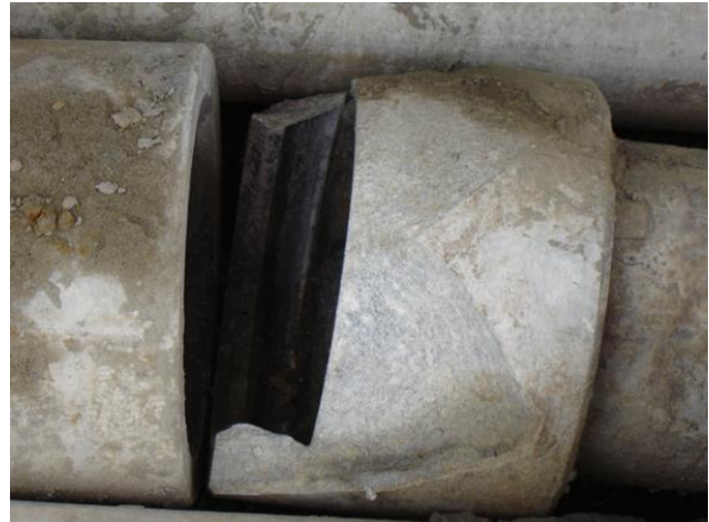
Figure 4-10. Asbestos cement pipe joint failure
