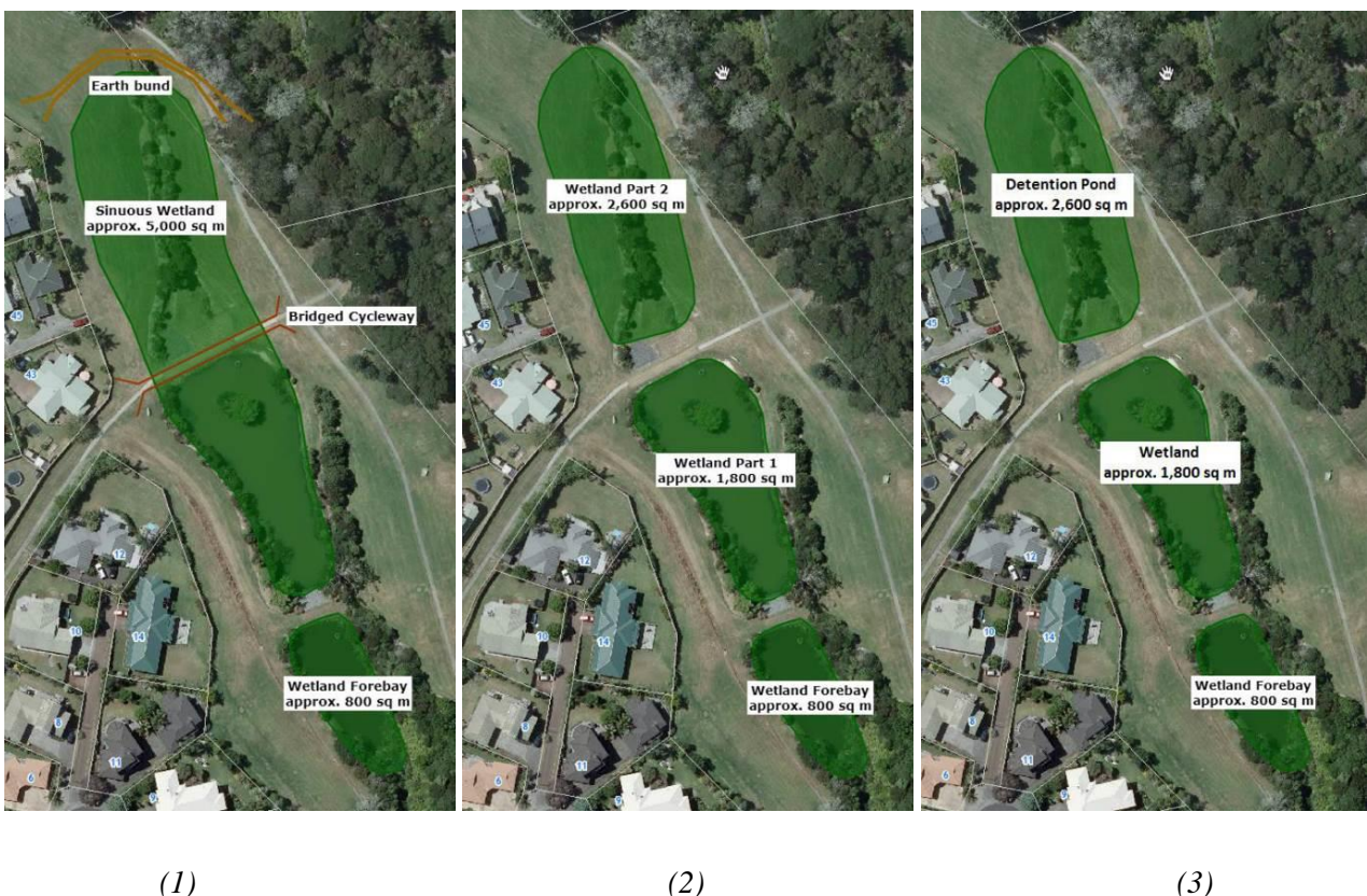
Figure 2: Layout of Unsworth Reserve Upgrade Options: (1) A Single Sinuous Wetland, (2) A Series of Sinuous Wetlands, (3) A Wetland and Pond in Series (Auckland Council, 2016).
