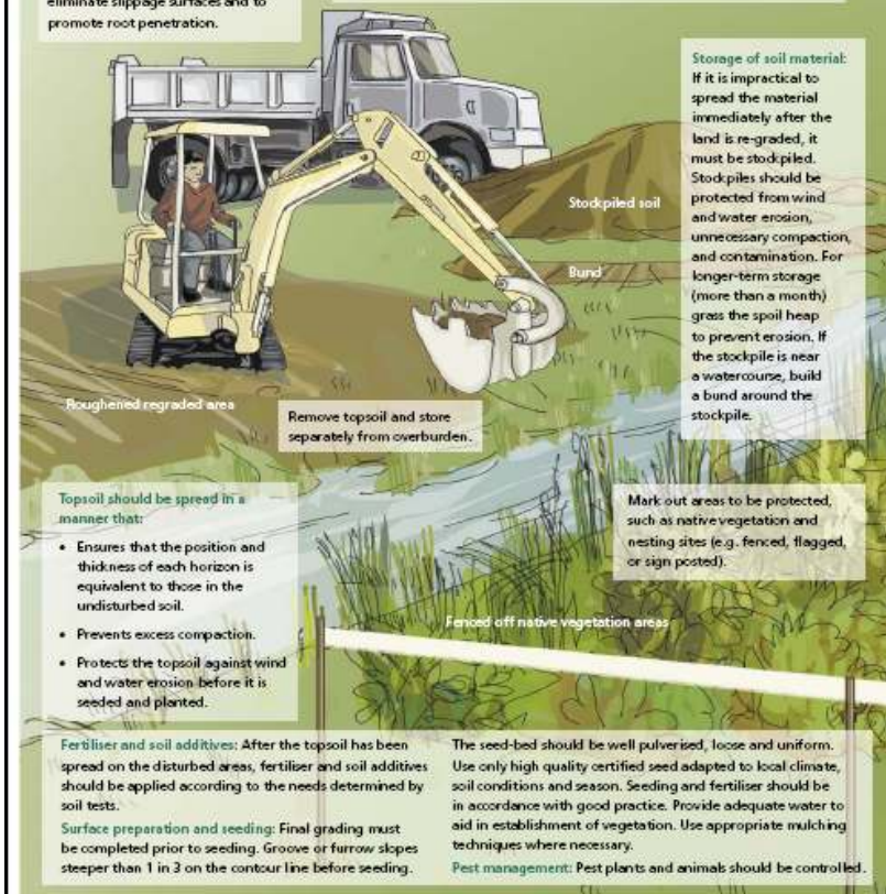
Sediment control and re-vegetation of drainage management work sites is often required to prevent soil erosion contributing to waterways.
