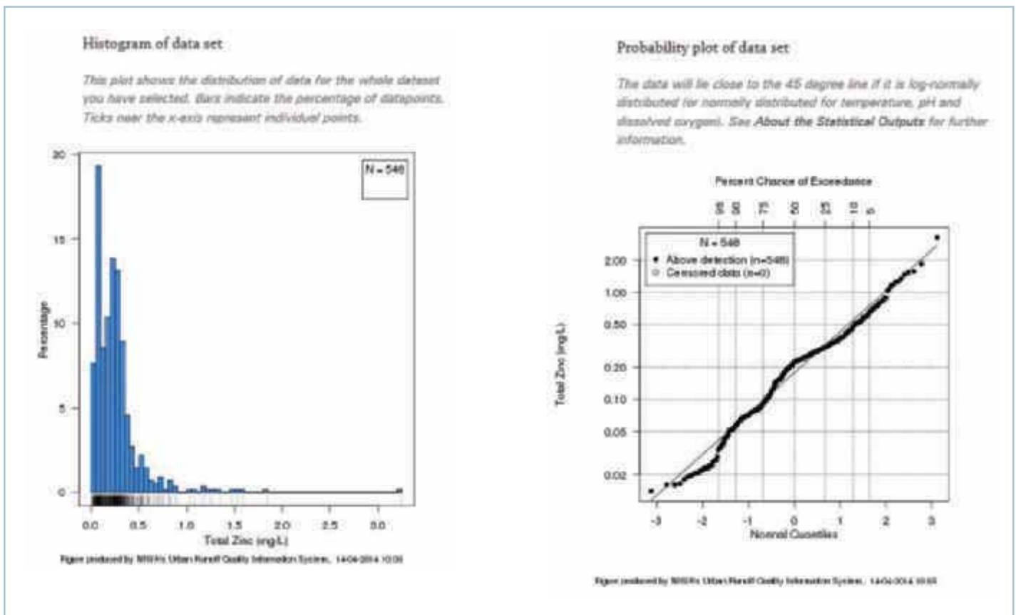
Figure 4 – Histogram and probability plots produced by URQUIS for TZN concentrations for samples taken from low density residential and CBD monitoring sites in Auckland for all water types and flow conditions
