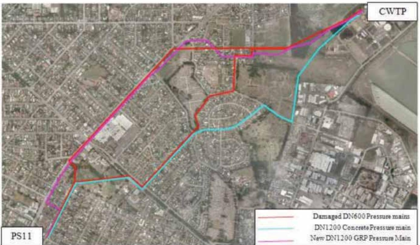
Figure 2 – Pressure Main 11 Alignments
