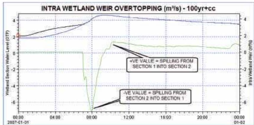
Figure 5 – 6.5 year rainfall record continuous simulation. Cumulative effect on reconfigured wetland water level
