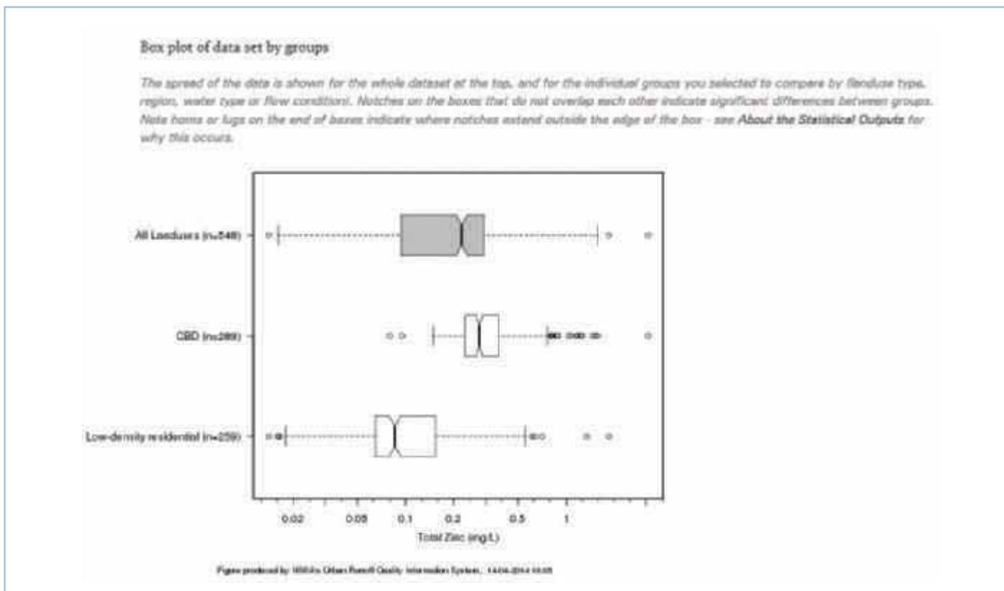
Figure 5 – Box plot produced by URQIS for TZN concentrations for samples taken from low density residential and CBD monitoring sites in Auckland for all water types and flow conditions
