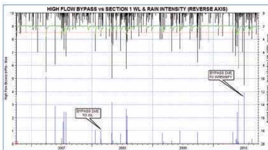
Figure 6 – four year rainfall record (2006 – 2010) – high flow bypass
