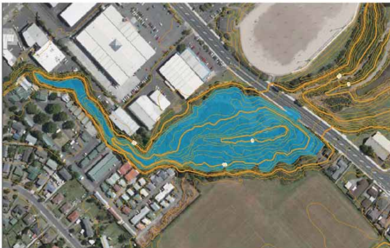
Figure 10 – Example depression extent with closed contours
