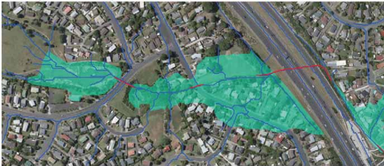
Figure 5 – Digitised culverts to adjust the DEM and corrected overland flow paths
