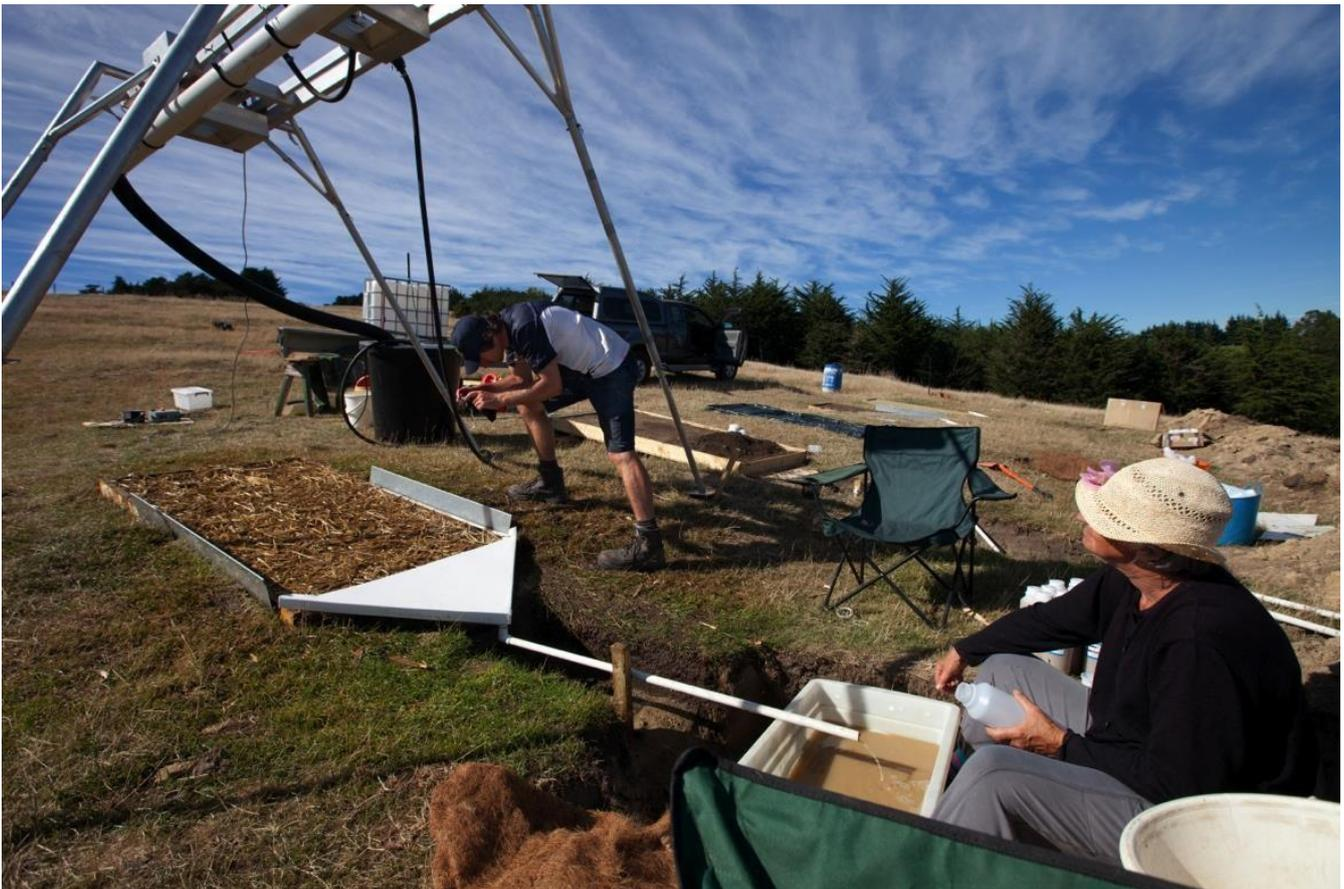
*Figure 3: Runoff plot and rainfall simulator setup for field experiments. Image © EOS Ecology.*
