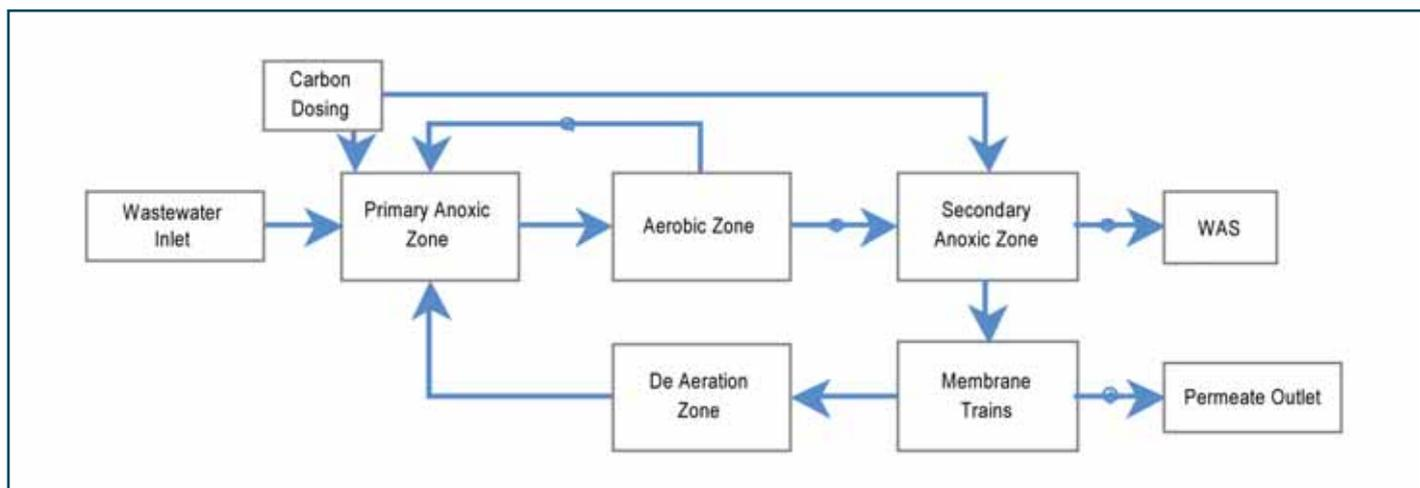
Figure 1 – Side Stream MBR Process Flow Diagram
