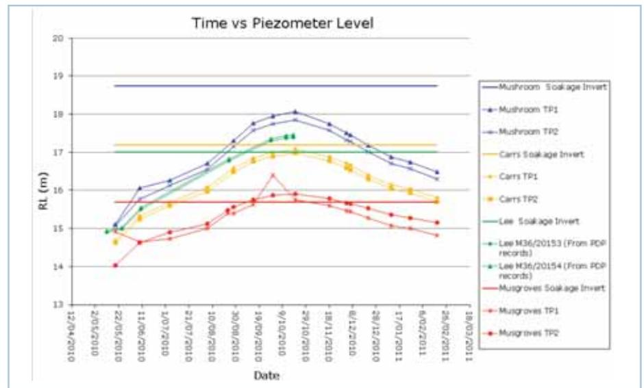
It can be seen from Figure 3 that as the design was progressing with assumed levels, the measured groundwater levels progressively approached, and in some cases exceeded, the designed soakage invert levels.
