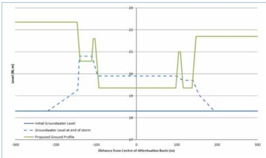
Figure 8 – Mushroom Basin modelled groundwater mounding at end of 3 year ARI (33% AEP) storm event with 2% AEP groundwater level (high groundwater sensitivity case)
