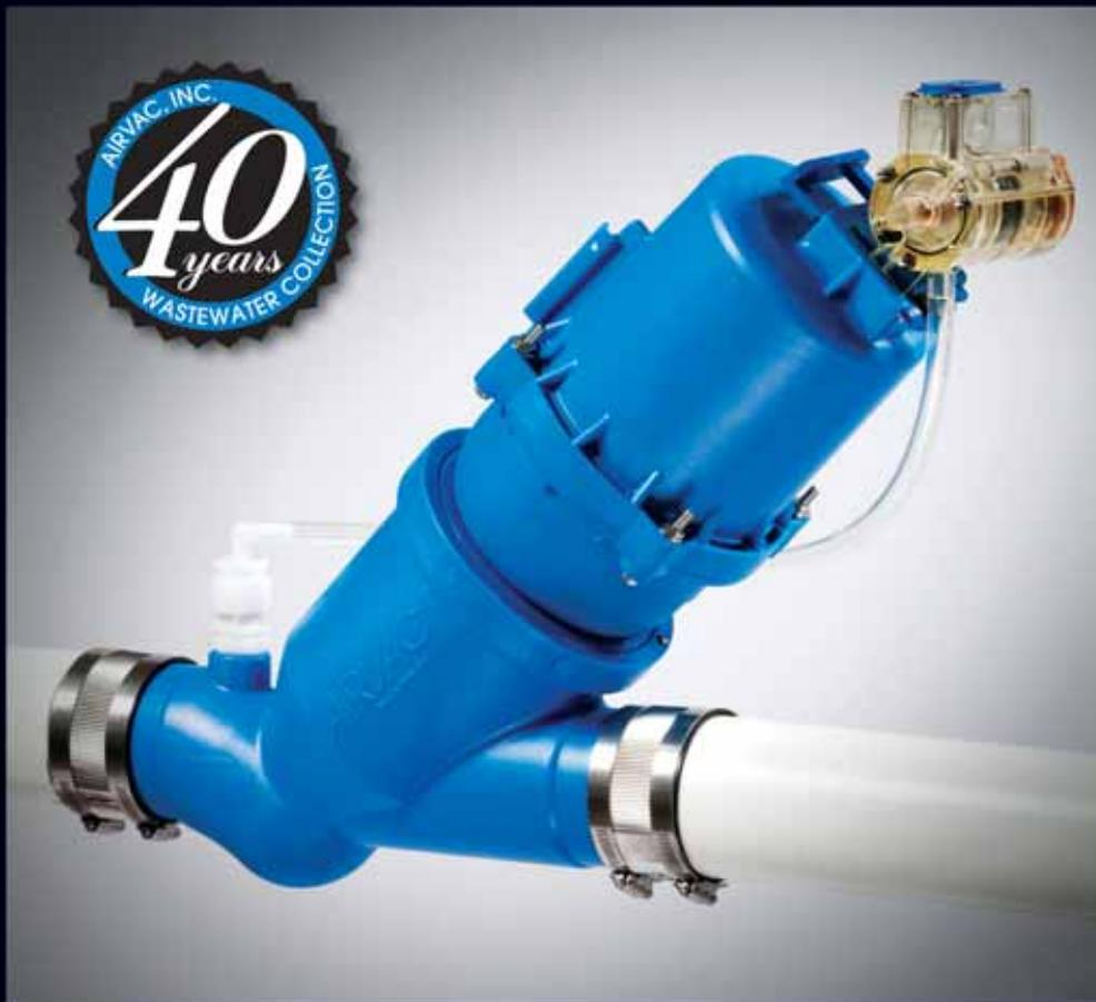
At the heart of every AIRVAC Vacuum Sewer System is the vacuum interface valve shown above. The development of this technology has made the advantages and flexibility of vacuum liquid conveyance possible. Although this valve represents our latest technology, many of our first valves are still in operation today.
