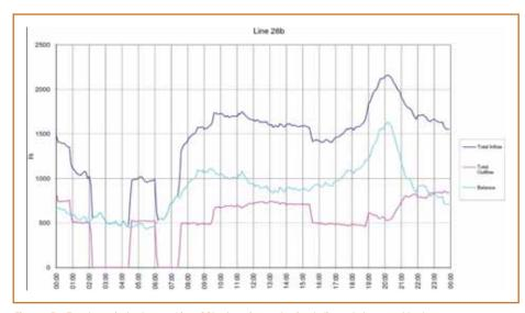
Figure 5 – Trunk main balance Line 28b showing a typical diurnal demand balance
