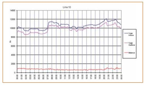
Figure 6 – Trunk main balance Line 10 showing effect of subtracting two large flows. Inconclusive result
