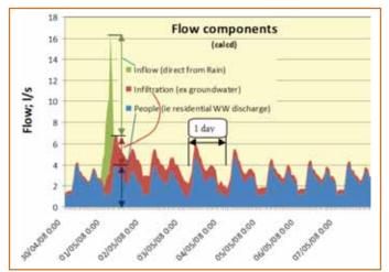
Figure 1 – Flow Components
