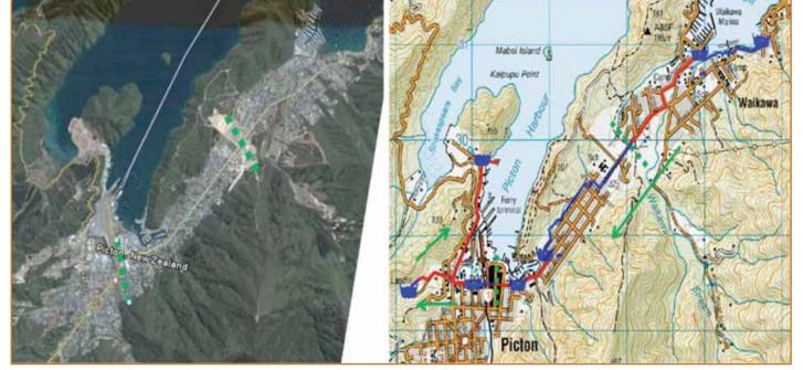
Figure 3 - Layout wastewater system Picton - Waikawa
