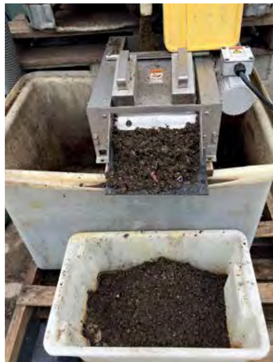
Top left: The new clog-free automatic liquid-to-solid KDS Waste Separator, Above: the more hygienic and easily handled output obtained in the Lord Howe Island application.
