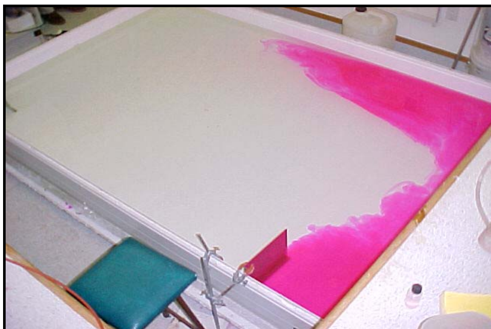
Figure 2-1 Tracer testing on a laboratory pond with 'stub' baffles
