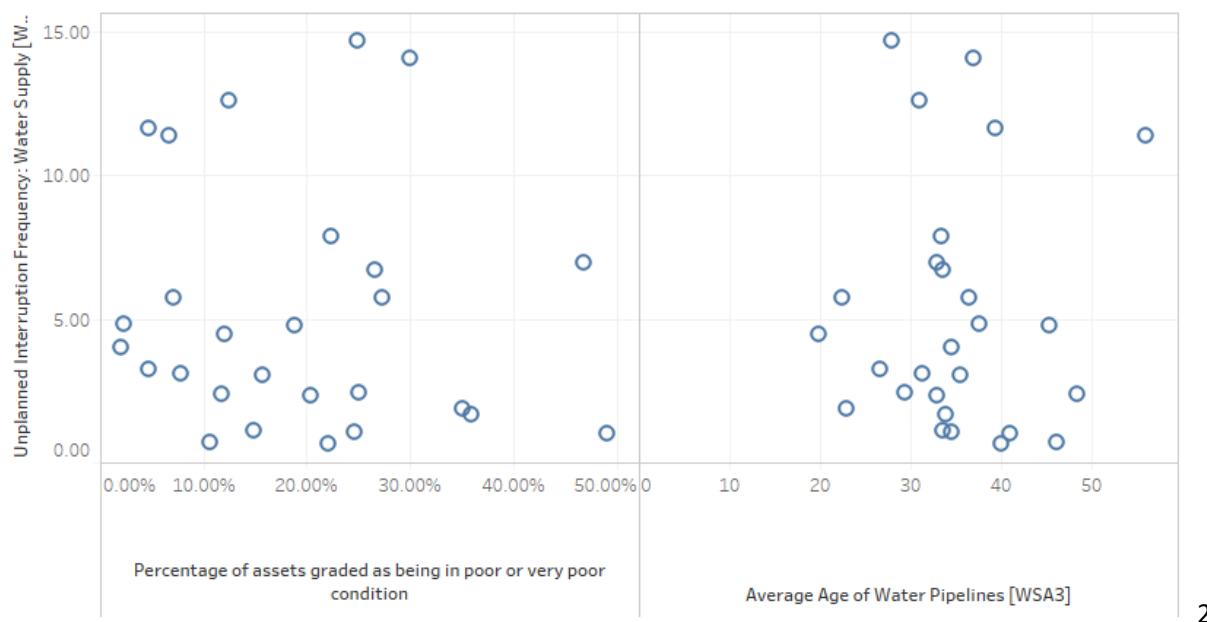
Figure 48: Unplanned interruption frequency plotted against water pipeline average age and proportion of assets in poor or very poor condition
