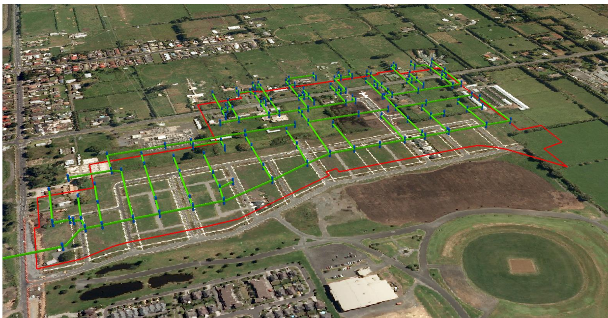
Figure 6: Study area (red line) and stormwater piped network (green lines) within the site
