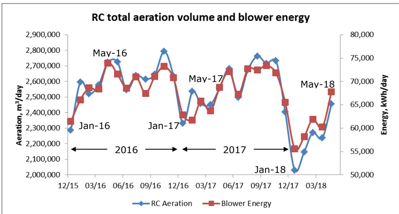
There was no discernible difference in sewage load characteristics year on year. Therefore, the aeration reduction observed is most likely due to the low DO control strategy implemented and reactors carrying a lower inventory in order to promote nitrite shunt.
