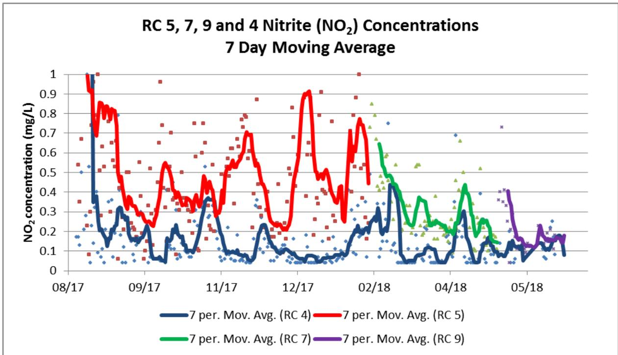
Figure 11: Reactor effluent nitrate concentrations for RC 5, 7, 9 and 4 (control RC).
