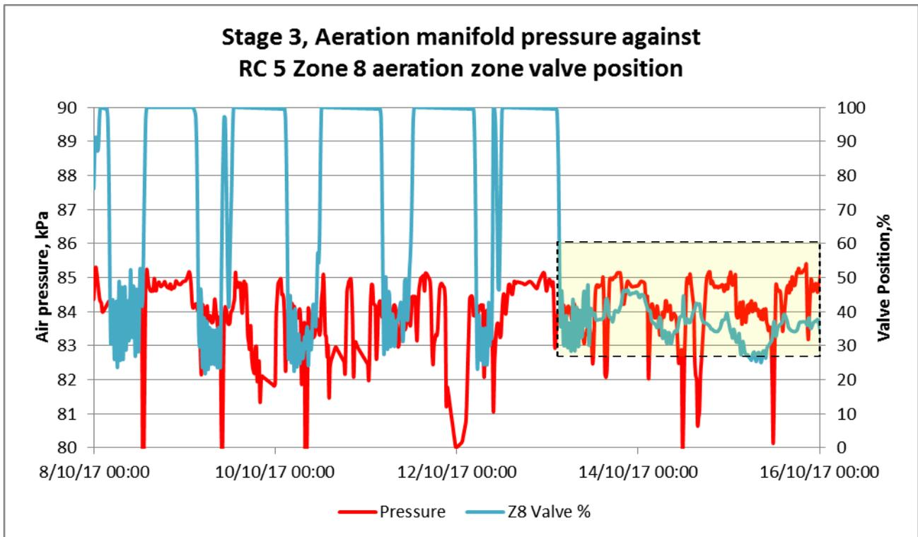
Attempts to measure savings in aeration could not be made due to technical difficulties with a newly installed air flow meter. The air flow meter installed on RC 5 was intended for the typical flow range. Due to the low DO mode operation, the air flow was under the low flow limit of the meter.
