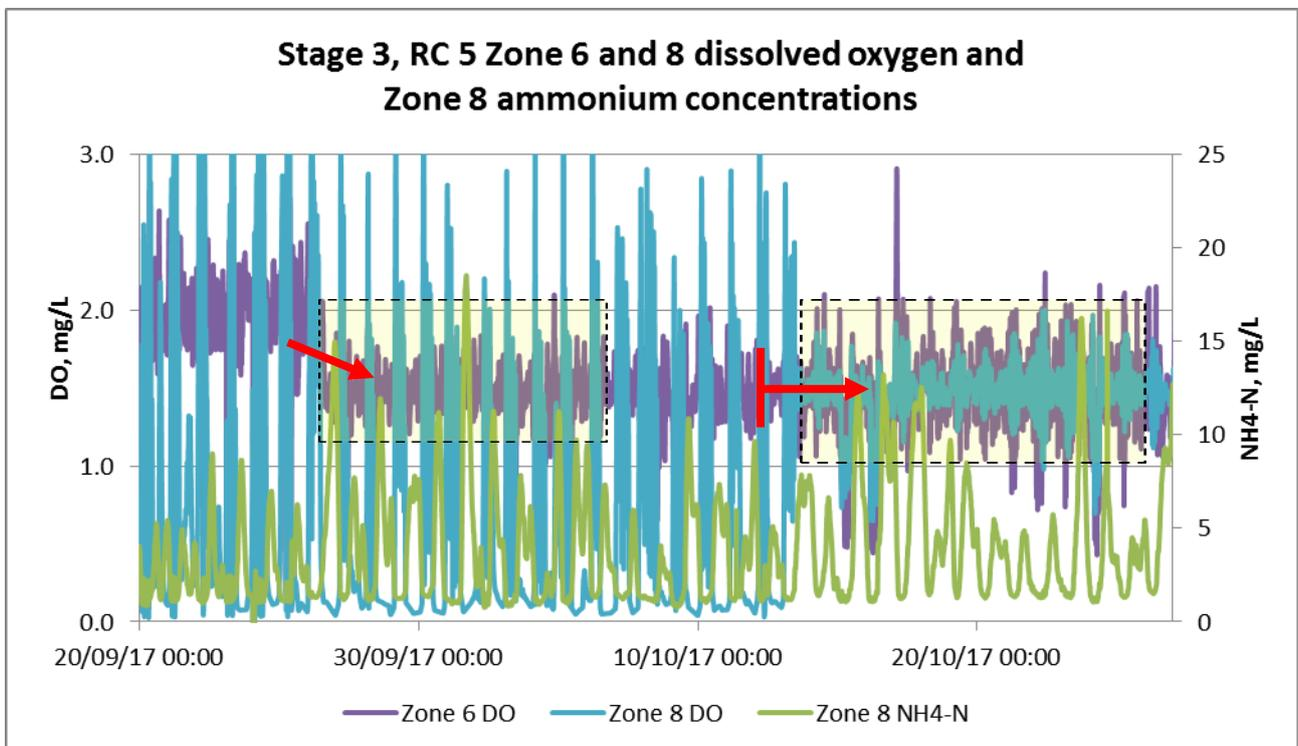
No distinct pattern could be observed in relation to impact of valve modulations on blowers' manifold pressure but a clear improvement could be seen in Zone 8 in terms of valve operation (Figure 8). Based on the DO trends it was concluded that the control regime had improved and valve modulation on RC 5 did not impact the blowers' manifold pressure.
