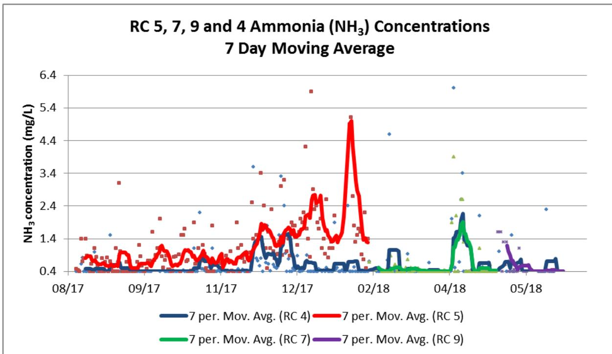
It can be seen that nitrite levels were overall higher and nitrate concentrations were lower in RC 5, 7 and 9 compared to RC 4 (control reactor). Slightly elevated ammonia levels were observed in RC 5. This is another factor which can promote nitrite shunt. Maintenance of residual ammonia allows aerobic AOB growth rate to be close to the maximum (Pusker Regmi, 2015). However this was not observed in RC 7 and 9. The reason is still being investigated.
