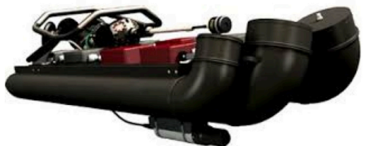
Figure A2.4 – Pipe Inspection float system, transporting in this example rear facing VPTZ camera, laser profiling and Sonar equipment below (MSI HD System, Photo Credit Red Zone Robotics)
