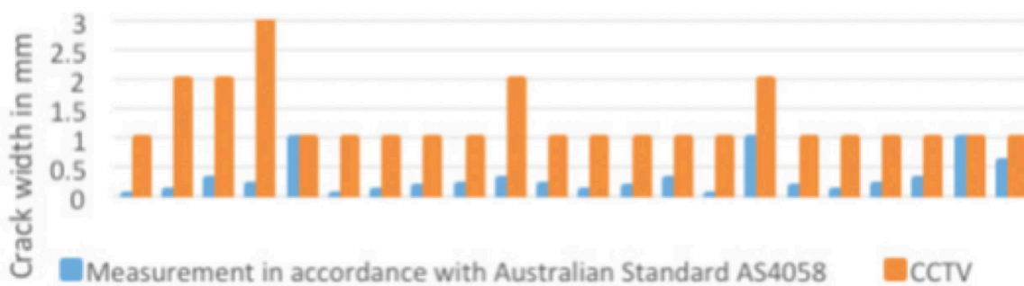
Figure C1 – Results of CPAA study comparing estimated widths of crack from CCTV inspection against actual width measurements
