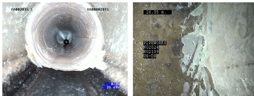
Figure D6 – Examples of extruded resin from a CIPP patch
