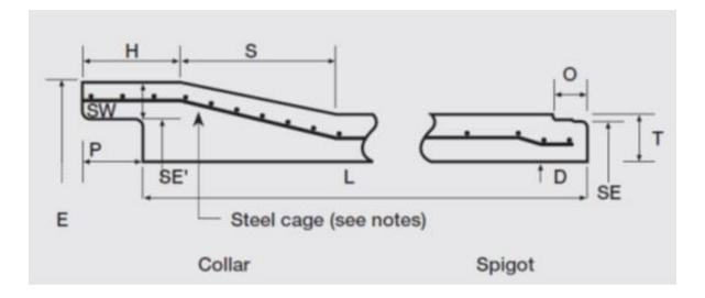
Figure 1: Long Section in Typical Reinforced Concrete Pipe
