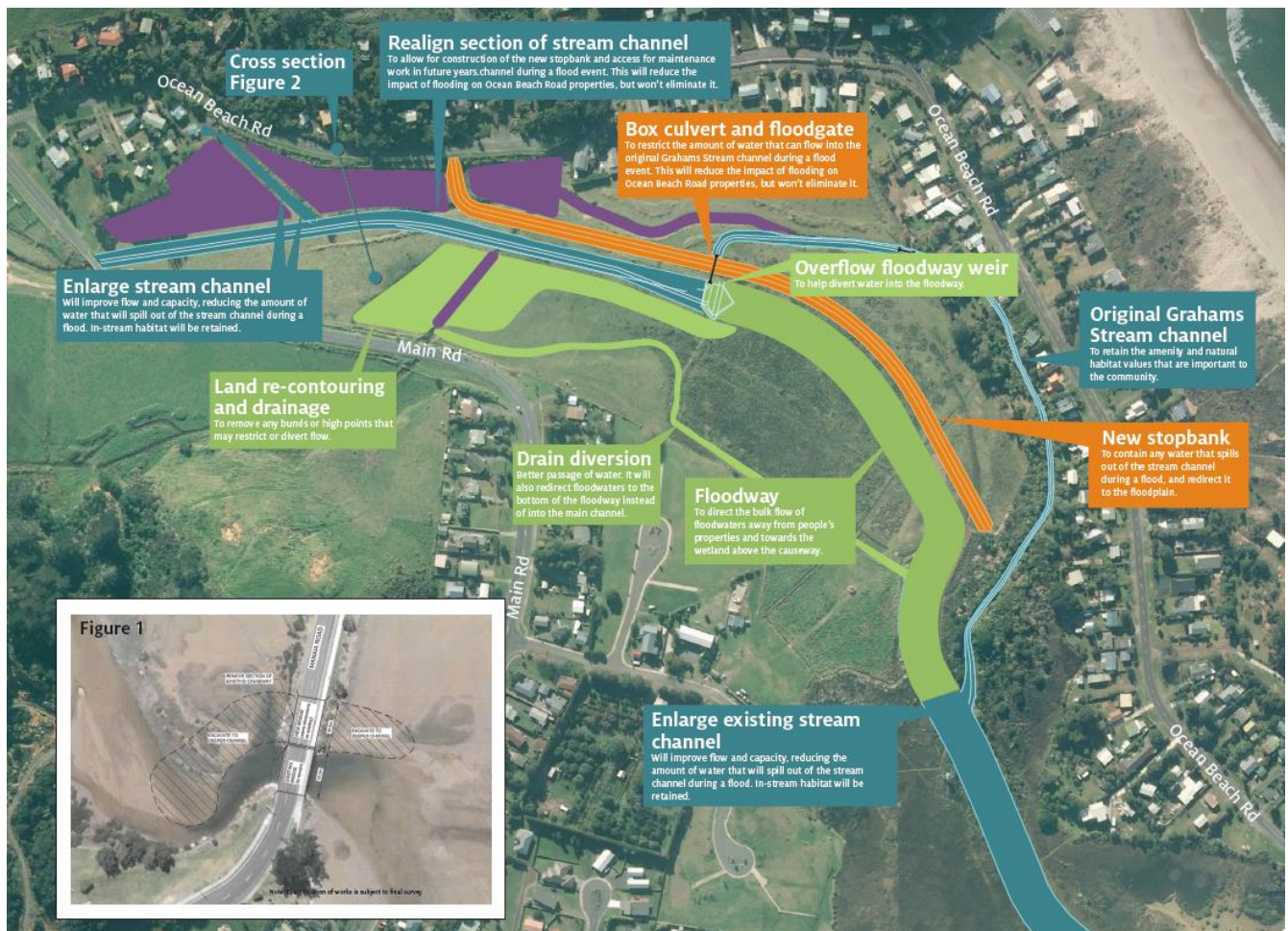
Figure 8: Schematic of flood alleviation components including stopbanks, increased channel capacity, floodway, floodgate, and redirected drain
