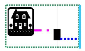
Customer Connection Sewer Property Connection Sewer Wastewater Reticulation Main Property Boundary Connection Point
