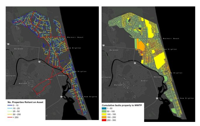
Figure 5: Example of output from assessment of asset criticality, pipe fault index as applied to an eastern area of Christchurch (Beca study completed for Christchurch City Council)
