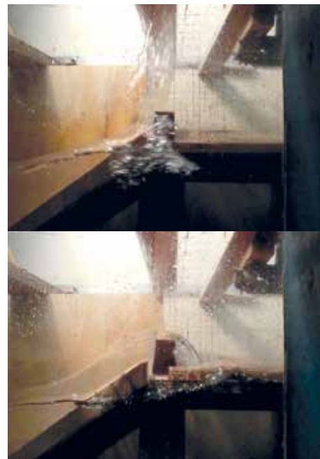
Figure 3: Examples of the 'white water' (above) and 'green water' (below) overtopping wave impacts.
