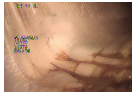
Staining in invert/wrinkles of the 'lateral leg' of the LJR from flow down the lateral.
