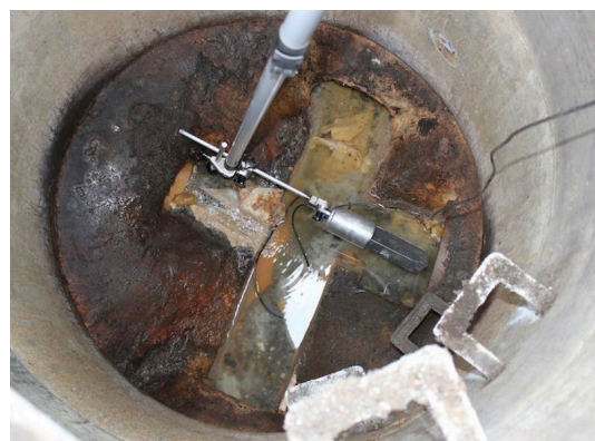
Figure A2.9 – SewerBatt inserted into the pipe for rapid inspection (photo credit Lanes Group plc)
