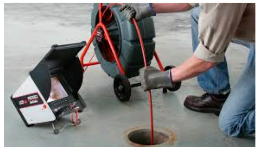
Figure A2.3 – Semi-rigid cable is used to push and pull the camera through the pipe
