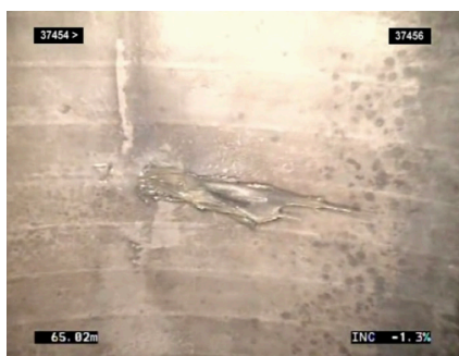
Figure D2 – Examples of vacuum and impregnation patches in CIPP liners
