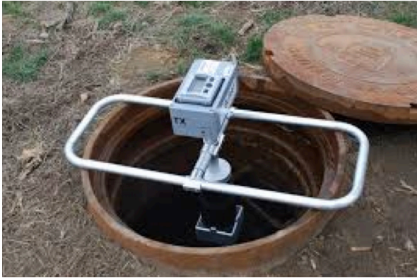
Figure A2.10 – SL-RAT device is positioned at each end of a pipe section to be tested (photo credit www.kci.com )
