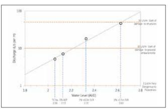
Figure 4: Modelled mean overtopping flows relative to water level and compared to tolerable flows
