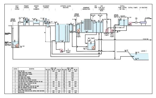
The construction team noted that the depth of the ASR and MBR structures would require extensive temporary works in poor ground conditions. Reduction in the depths of these structures would result in reduced risk and costs during construction.
