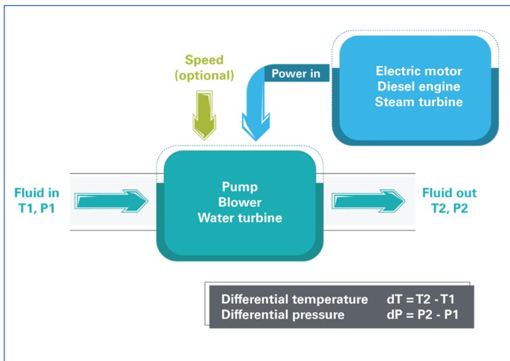
For multiple pumps operating in parallel, pump efficiency and flowrate are able to be measured simultaneously for individual pumps using the Thermodynamic method.
