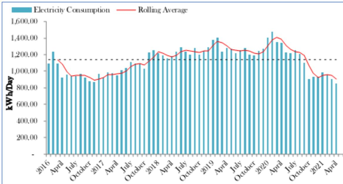
Pharazyn pump station had been increasing in electricity consumption for the previous four years, while the pumps were operating outside of their POR. Beginning in 2020 this trend sharply reversed and the electricity cost savings were due to replacing the existing 130 kW pumps with 160kW pumps which were operating at their BEP.
