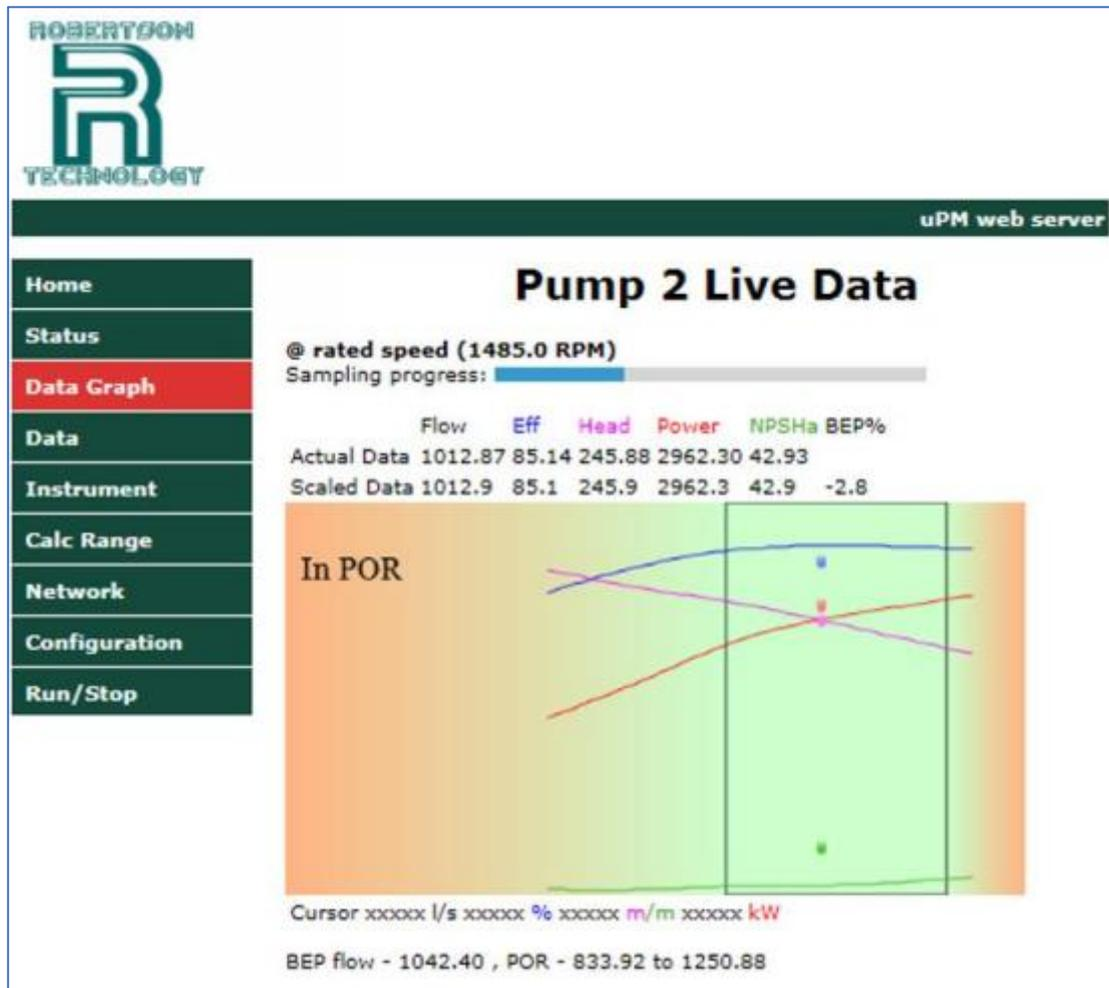
Advanced features of the MicroPM Pump Monitors include station level pump scheduling functionality where it advises the user which pump combinations and VSD speed set points would provide their demand flow rate requirements in the most efficient and cost-effective manner.
