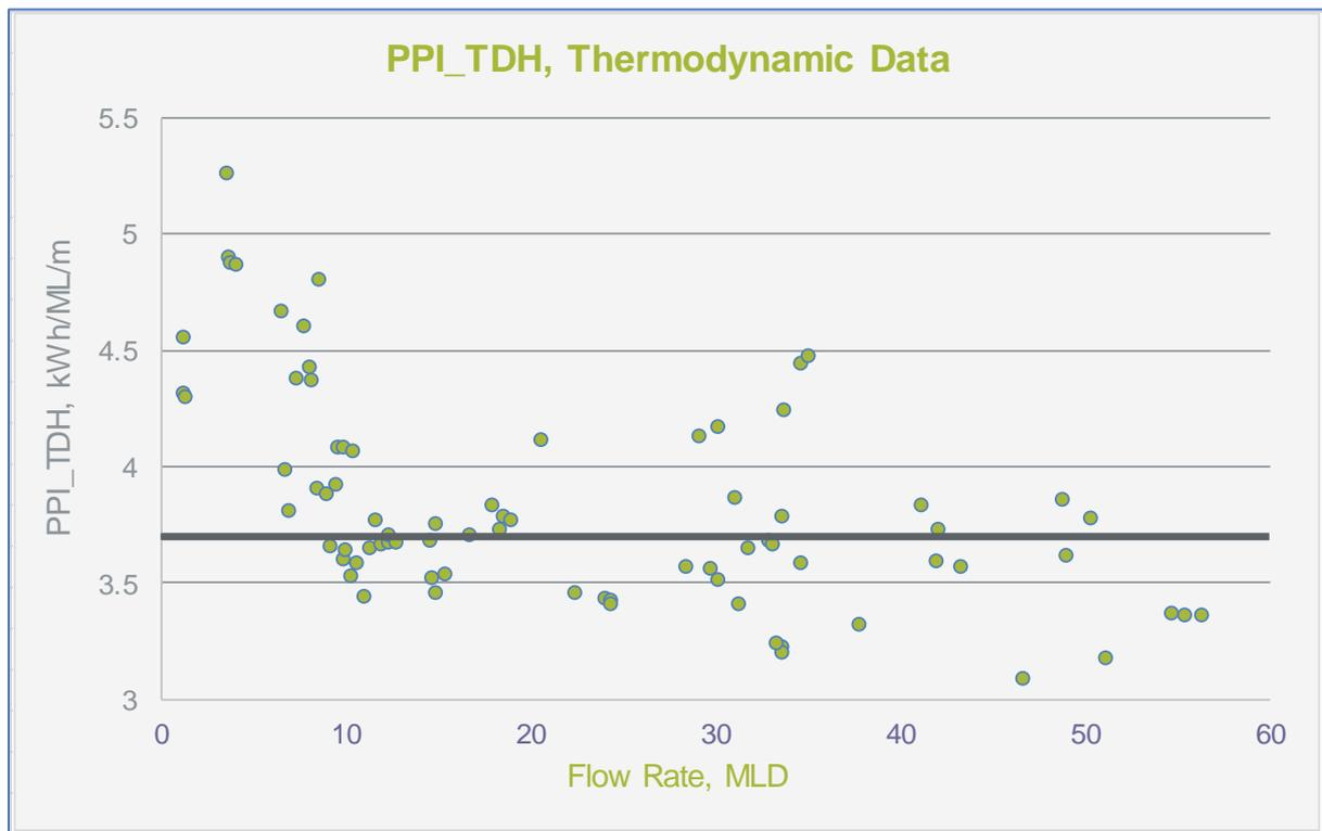
PPI\_TDH efficiency values in the database vary from 3.1 to 5.3 kWh/ML/m and a value of less than 3.7 is defined for when a pump is operating efficiently, based on the 50th percentile of the database. If the PPI\_TDH exceeds the 75th percentile, in this case a value of 4.1, potential electricity cost savings or operational efficiency improvements might exist for the particular pump and further analysis is recommended.
