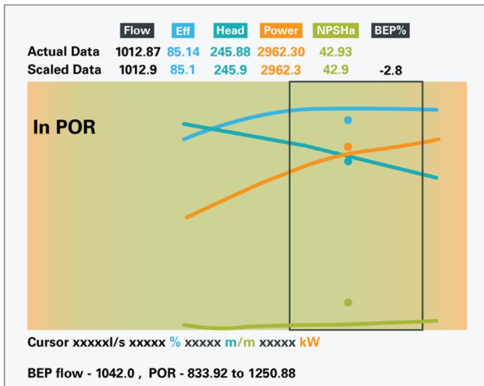
Figure 7 shows an example of how ensuring the pumps operate within their POR realises electricity cost savings.
