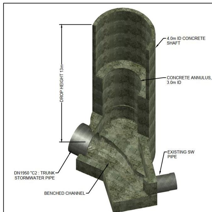
The approach pipe is a DN450 concrete pipe with a design flow of 375  $\ell/s$  in the 10% annual exceedance probability (AEP) storm. The drop height is 13 m from the invert of the proposed incoming high-level pipe to the floor of the shaft.
