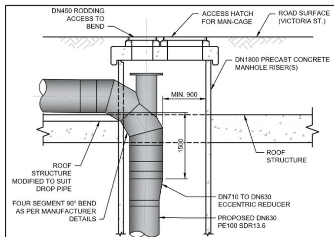
Hydraulic design for the counter-current arrangement indicated the pipe exit velocity would be around 6 m/s, so abrasive wear of a concrete splitter block and curved baffle may occur. Stainless steel was selected to provide appropriate wear resistance in this location. Given the inherent wear resistance of PE, rapid abrasive wear was considered unlikely; however, the bend at the base of the chamber was increased to SDR11 for added risk mitigation.
