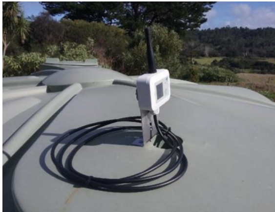
Figure 10.1: Loosened sensor cable coils due to weather conditions.
