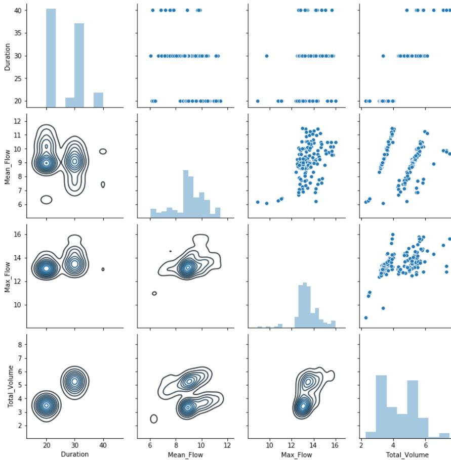
Figure 13 Use of data visualisation to identify the characteristics of dual-flush toilet events.
