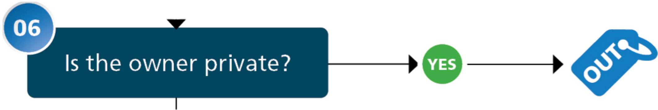
Query also identifies and 'tags' private pipes  $\geq 300\text{mm}$  for double checking
