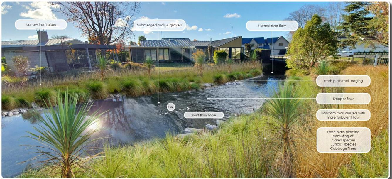
Figure 9 – Visualisation of the finished riffle used to assist with consultation in the early stages of the project
