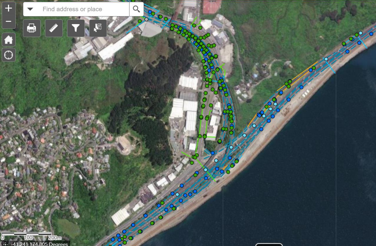
Example: Ngauranga Interchange (Wellington): Stormwater asset features
