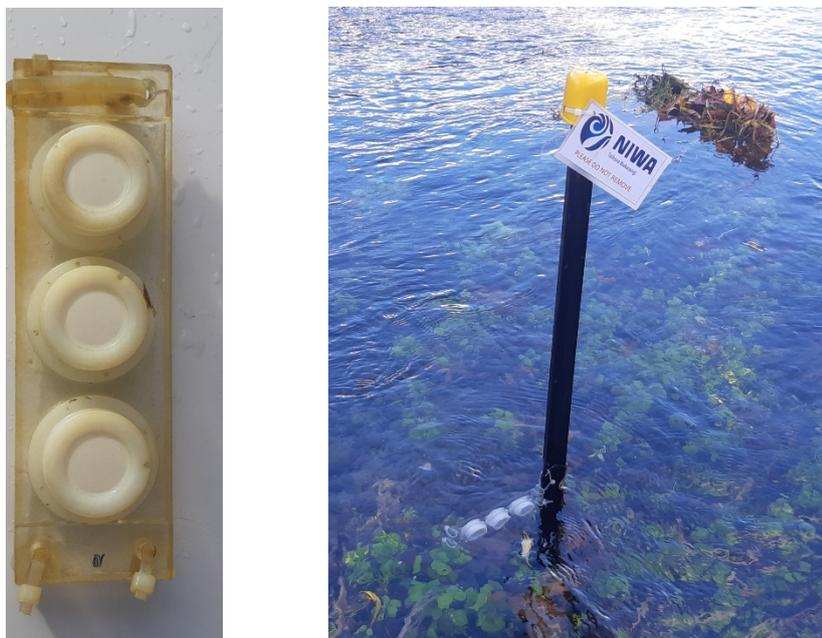
*Figure 5-1: DGTs deployment methods. Left: DGTs contained within an acrylic plate holder. Right: Instream deployment with acrylic holder attached to waratah. Left photo taken after deployment.*
