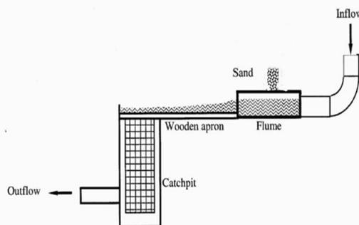
Figure 7: Laboratory Performance Testing Set up
