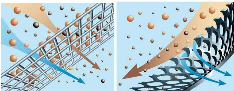
*Figure 2: Illustration of direct (left) and indirect (right) screening: source CDS technologies*
