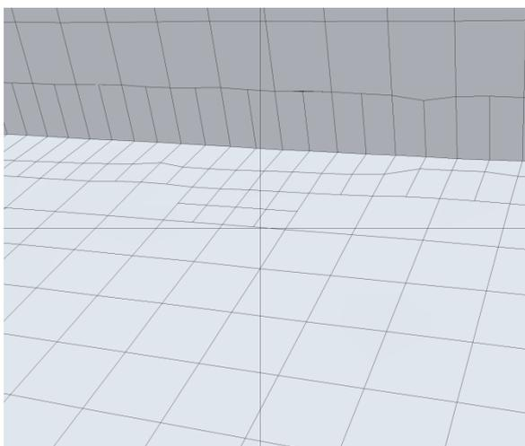
*Figure 3. Trimmed hexahedral mesh changing mesh size to account for changes in geometry*
