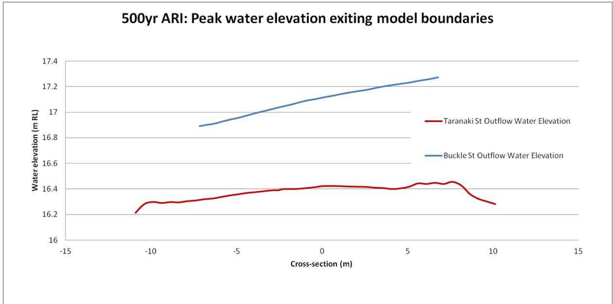
Figure 9. Geometry 2 500yr ARI peak water elevation of flow exiting model boundaries, see, Figure 10 for cross section locations
