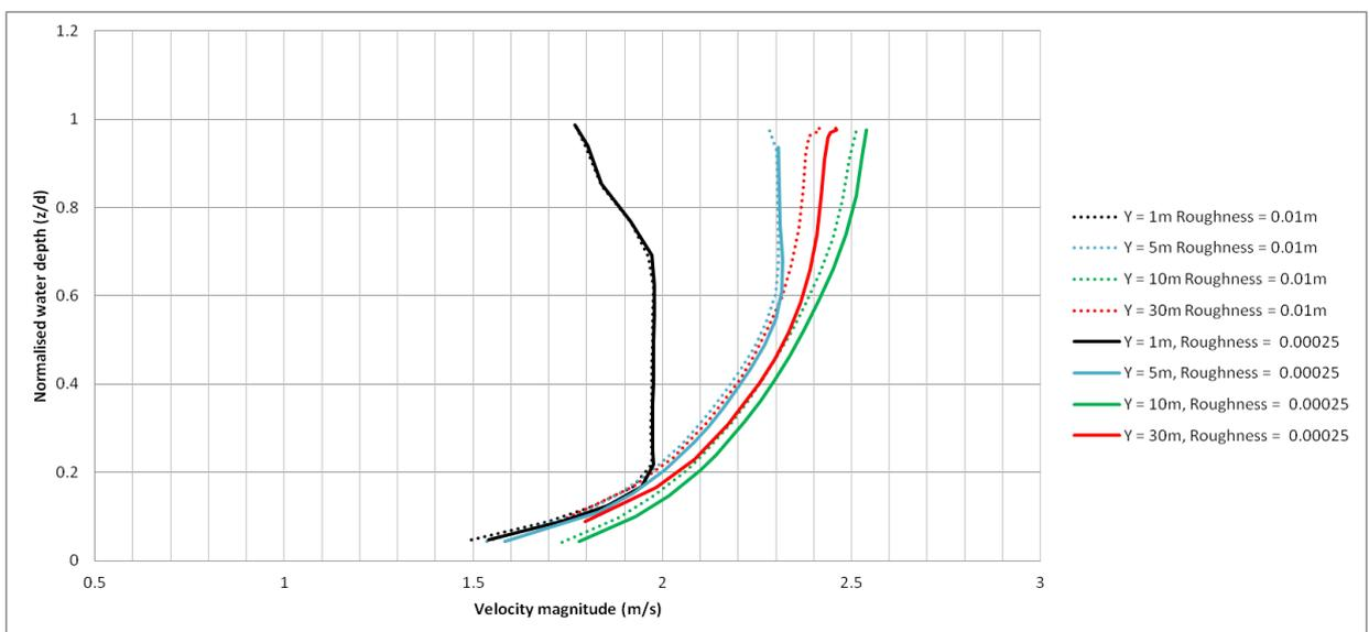
Figure 6. Velocity profiles taken at 1 m, 5 m, 10 m, and 30 m downstream from the Taranaki St model boundary. Profiles taken from the 500 yr ARI model, with floor roughness height at 0.01 m and 0.00025 m
