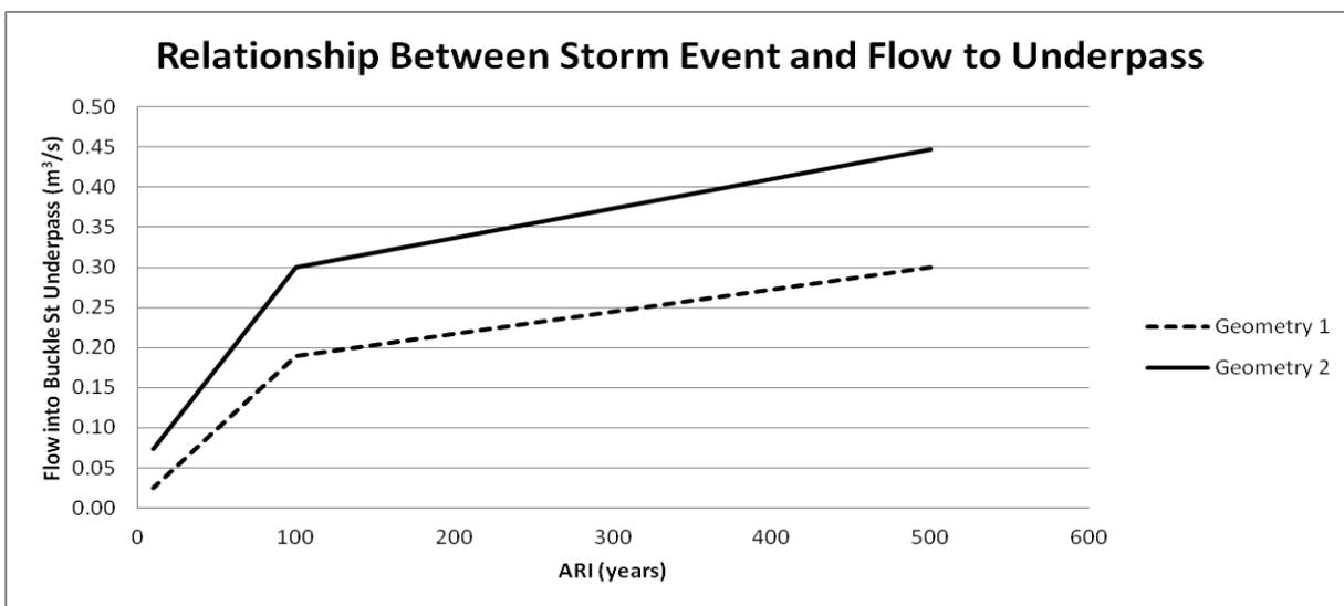
Figure 7. Relationship between storm event and peak flow to underpass
