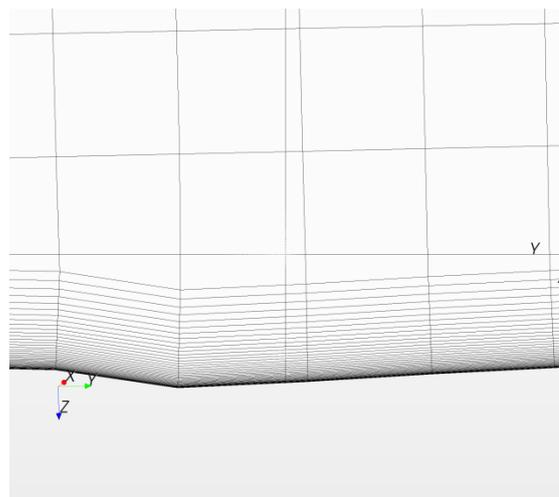
*Figure 4. Prism layer creation: Refinement of mesh close to the floor of the model*
