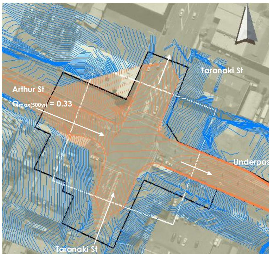
Figure 1. Site layout and source data, where the orange contours show the 0.05 m contours of the new road alignment, blue contours show the 0.05 m contours of the existing land surrounding the intersection, black shows the area of interest and white shows the final model extent which was chosen to minimize model surface area.
