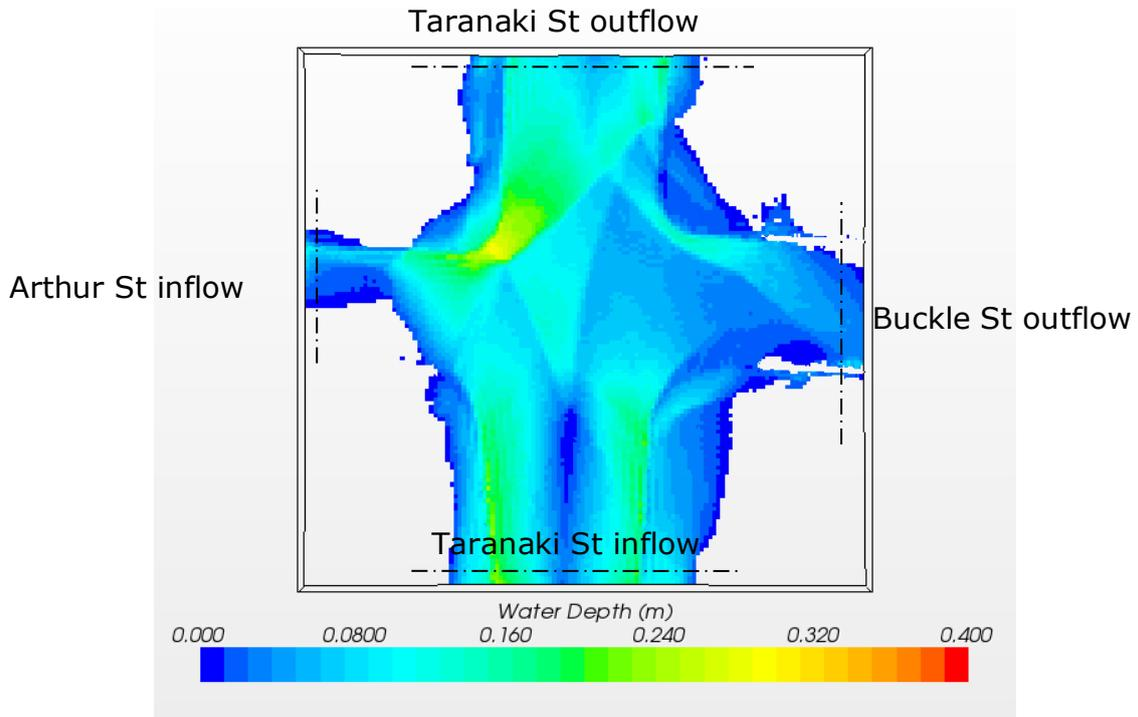
Figure 10. 500 yr ARI peak water depth, showing Figure 8 cross section locations
