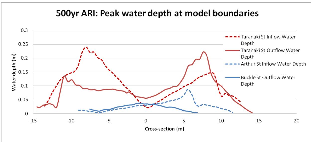
Figure 8. Geometry 2 500yr ARI peak water depth at model boundaries, see Figure 10 for cross section locations
