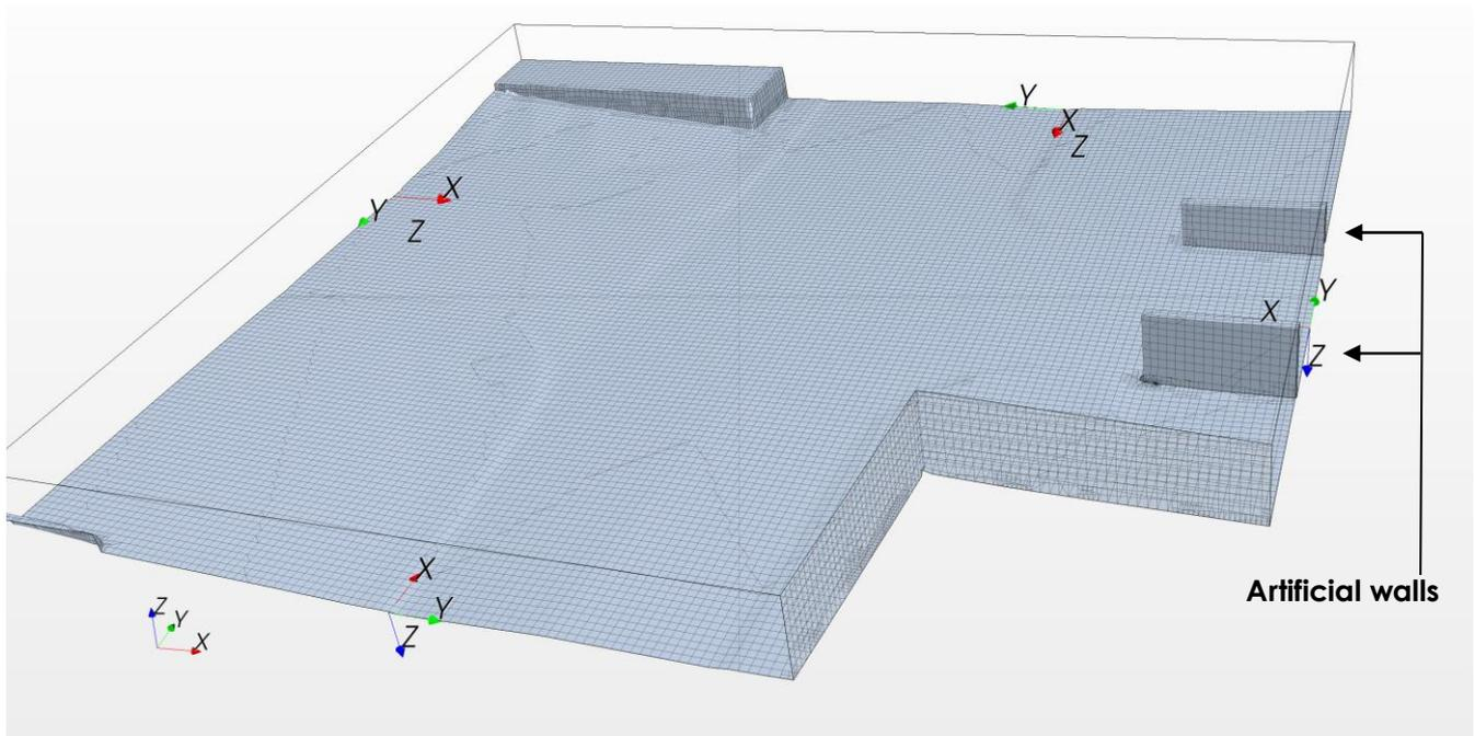
*Figure 2. Model mesh: The walls and road surface as represented in the model. These surfaces represent the bottom and side of the mode that contain the simulated flow. Artificial walls at the tunnel entrance were used to overcome unacceptably high roughness from the design data at these locations.*
