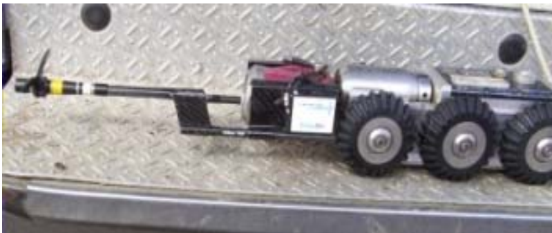
Profiler mounted on CCTV Camera
