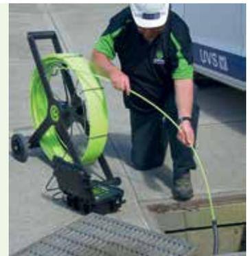
**SewerSerpent225 can be operated by one person for fast scans of sewer laterals to rapidly identify leaks and inflow sites**
