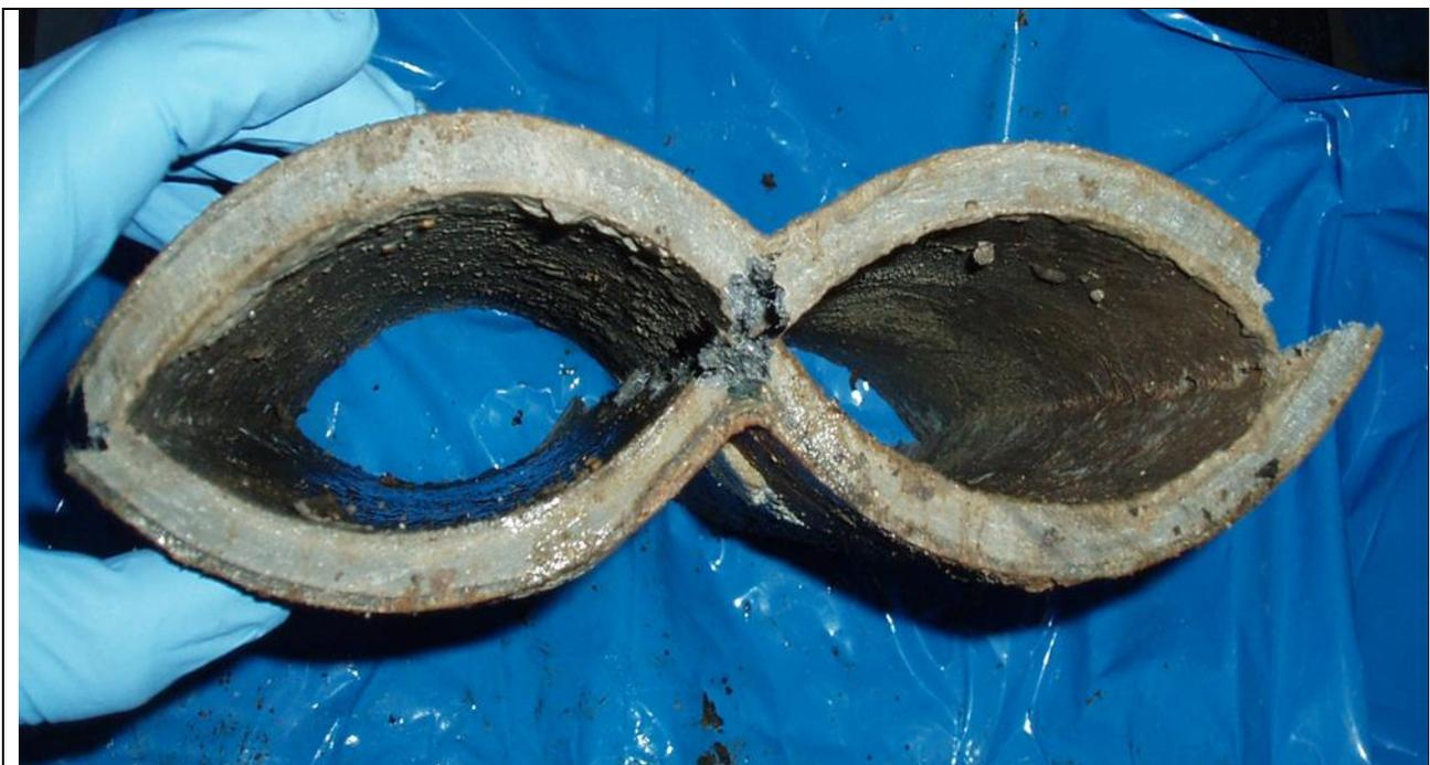
Figure 1. Asbestos cement pipe sample after crush testing. This illustrates how a fractured rigid pipe can hinge about the four breaks to behave as a flexible pipe.
