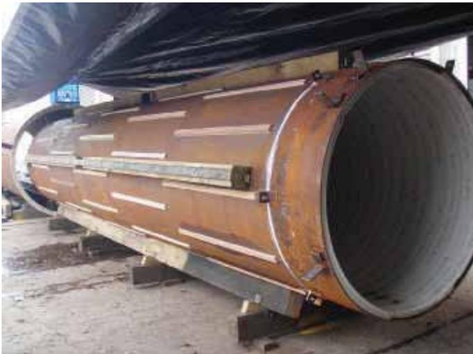
Picture 6 – Slots in the steel tube covered while the liner is grouted. The covers were removed prior to it all being inserted into the pressure vessel for testing.
