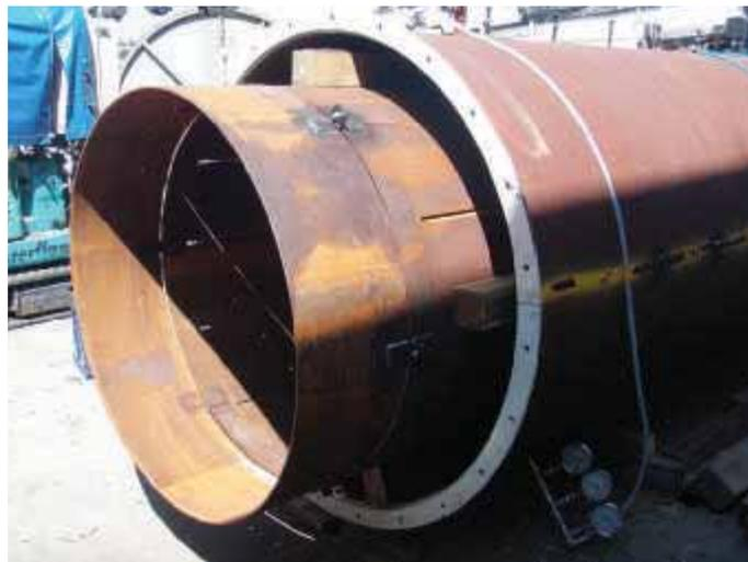
Picture 4 – Steel tube fabricated to support the Rotaloc liner to be wound inside it. Slots were cut in the tube to allow hydrostatic pressure to be applied to the liner.
