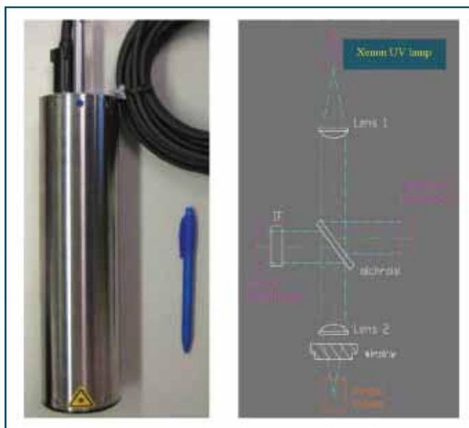
Figure 2 – UV-fluorescence OIW sensor and principle of its operation
