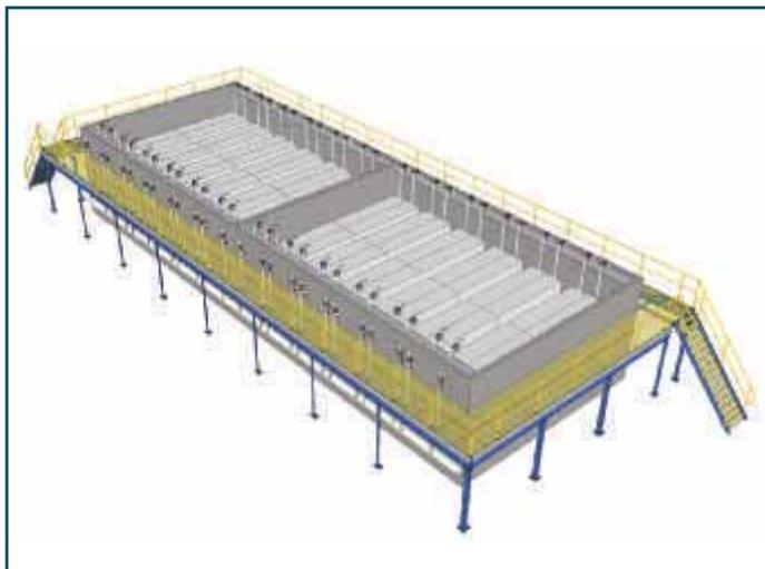
Figure 4 – 7,500m<sup>3</sup>/day MBR system derated to 4,500m<sup>3</sup>/day conservative capacity based on actual performance in an industrial application
