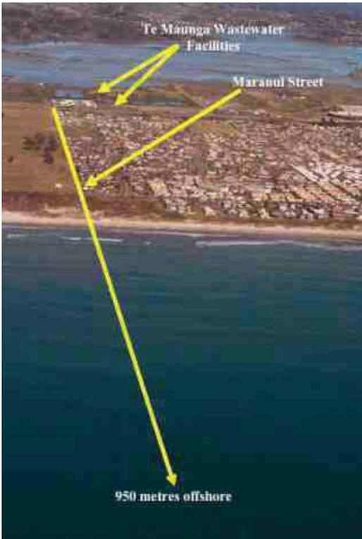
Line of landward effluent pipeline and marine outfall – Tauranga City photo
