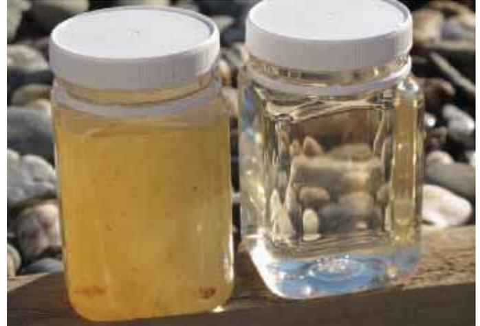
Figure 1 – Raw and treated water from an Apex Environmental MBR
